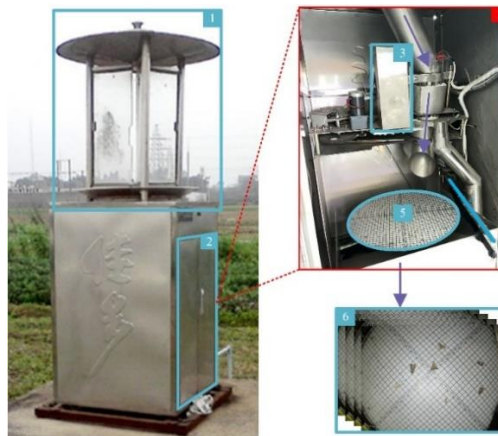
Figure 1. light-trap pest collection device. (1) Pest light-trap device; (2) interior structure; (3) camera; (4) pest cleaning device; (5) white background board; (6) original light-trap dataset.
