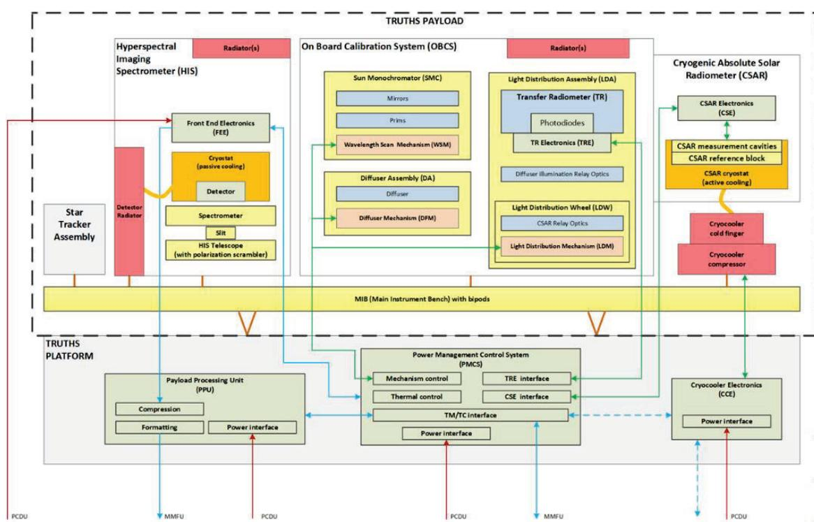
Figure 1: Payload architecture at the end of phase B1
