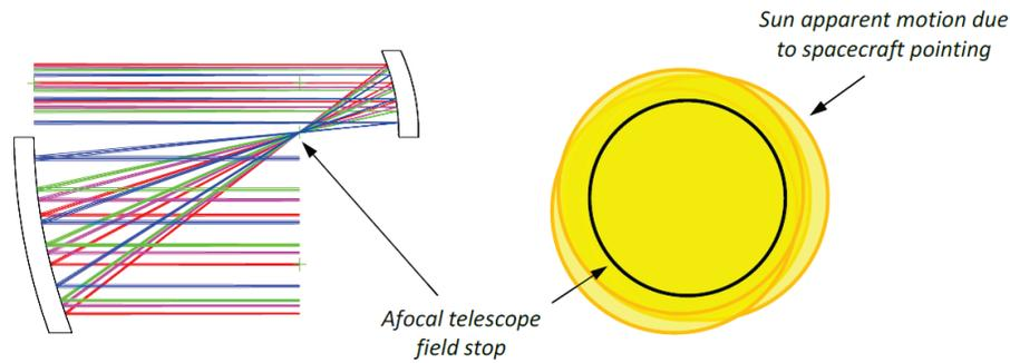
Figure 3: Implementation of afocal array field stop.
