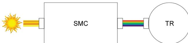
3. Measurement of the diffused radiance of the same SMC spectral output beam by the HIS and transfer radiometer.
