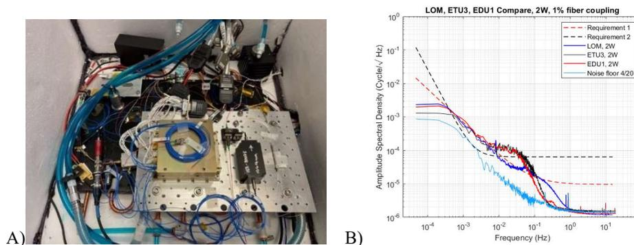
Figure 6 A) RF sideband phase noise measurement setup at GSFC, B) Measured RF sideband phase noise of different amplifier units.
