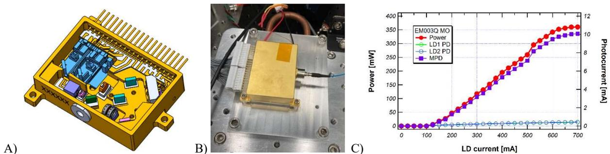
Figure 4 A) Internal design of the TRL 6  $\mu$ NPRO package. The fiber coupling assembly is not shown. B) Completed EMQ  $\mu$ NPRO package under test. C) Output power of EMQ  $\mu$ NPRO package. Photocurrents of internal photodiodes are also shown on the right axis.
