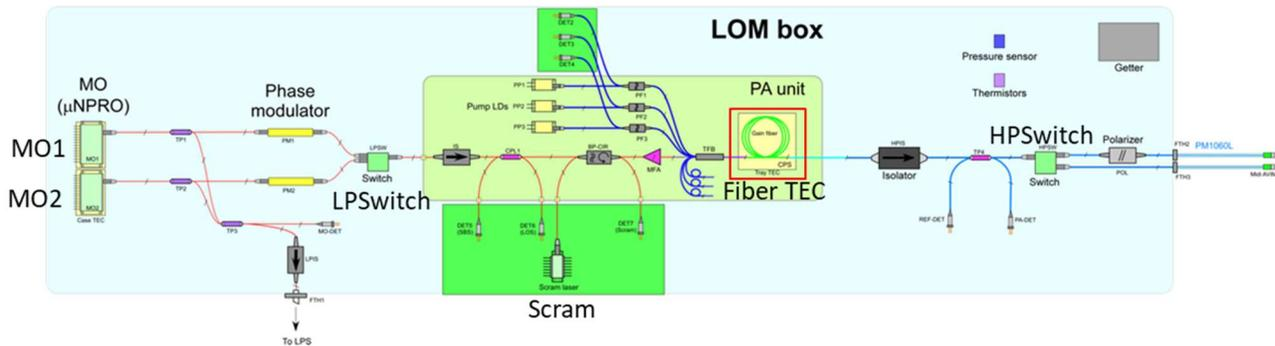
Figure 2: LISA TRL6 laser optical module optical layout.
