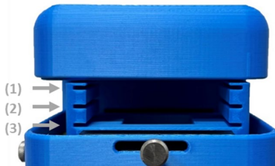
Figure 7. Three available slots for inserting a microscope slide or a cuvette.
