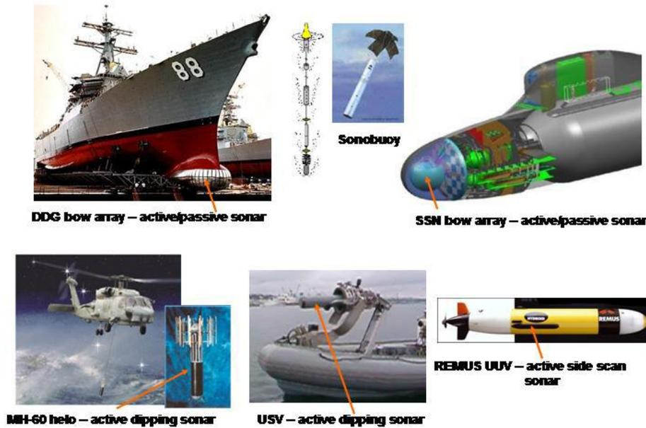
Figure IV. Example Undersea Sensors as Vessel Payloads
