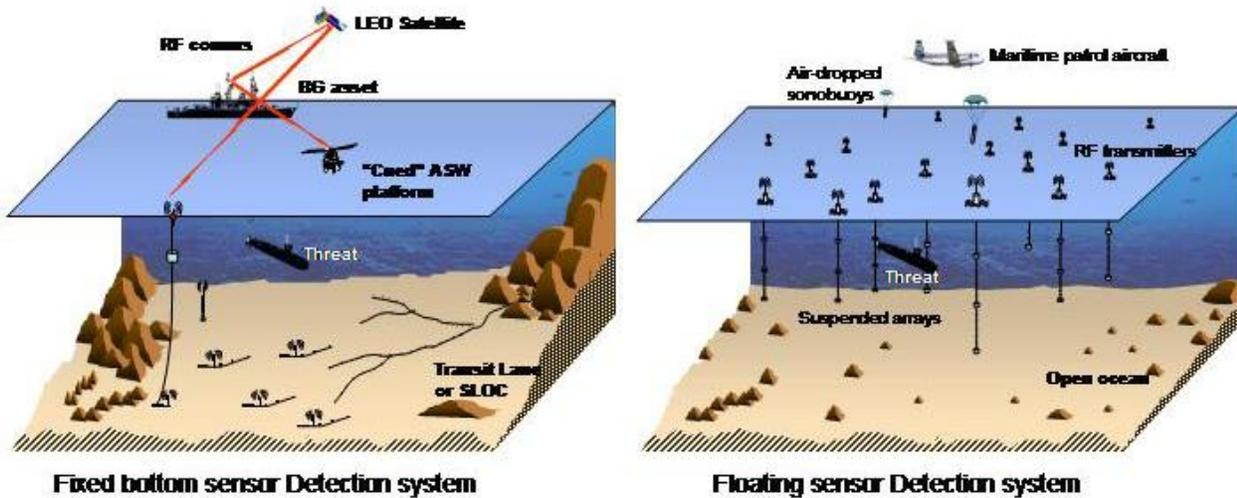
Figure V. Example Distributed Sensors Applied to Barrier Search
