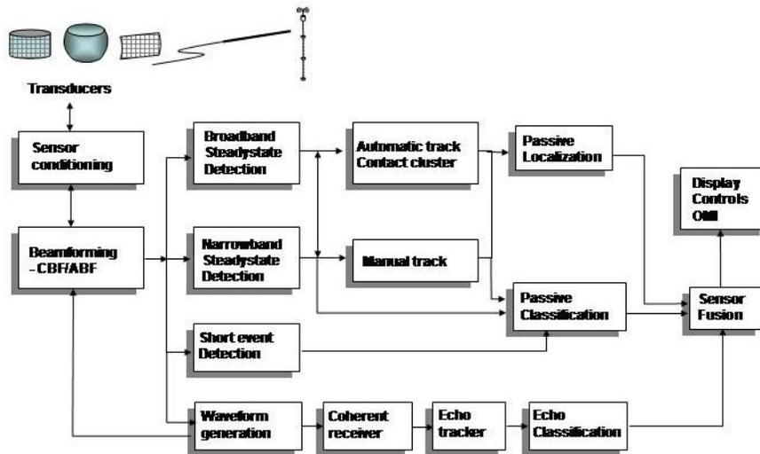
Figure XX. Canonical form for undersea sensor signal processing and automation
