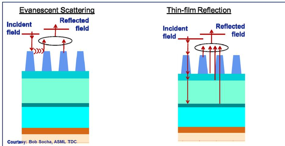
Figure 15: How to measure features much smaller than  $\lambda/NA$  with optics? Evanescent scattering and thin film reflection phenomena in scatterometry [41].
