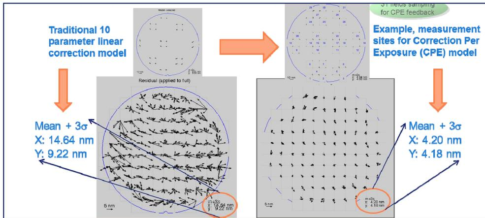
Figure 7: Higher order overlay correction model requires additional measurements.
