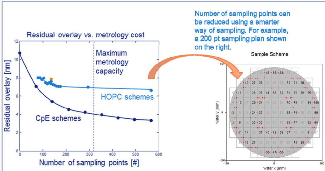
Figure 9: Overlay improvement is enabled through increased sampling and corrections per exposure.
