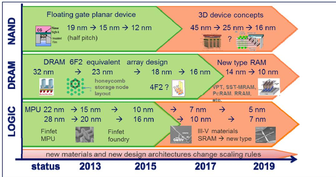
Figure 11: Device scaling assumptions as input for lithography solutions.
