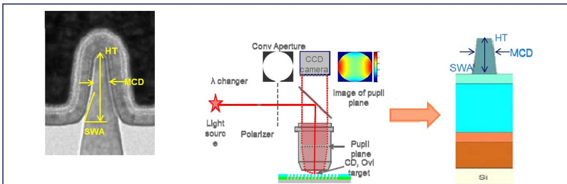
Figure 12: How to support the needs of new device structures? FinFET transistors need profile and height control in addition to CD [42].
