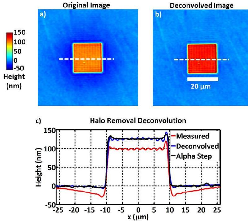
Figure 3: Halo removal using deconvolution with the OTF.
