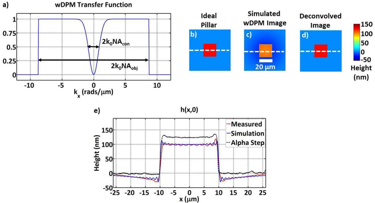
Figure 1: Simulation of DPM image formation using the optical transfer function.
