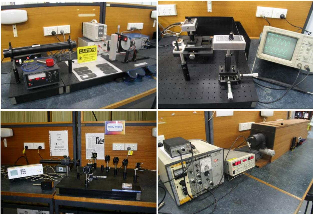
Fig. 2 Experimental setups for the Correlation interferometry (top), Polarisation and Berry phase (bottom left), and photon counting and interferometry (bottom right) experiments in the undergraduate optical physics laboratory, Department of Physics, Macquarie University. Photos: Dr Gina Dunford.
