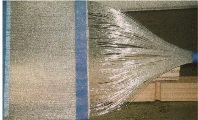
(b) Fiber optic panel for 2-D uniform light source component
