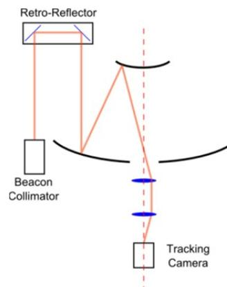
Figure 8: Alignment of Beacon Laser using a Retro-reflector
