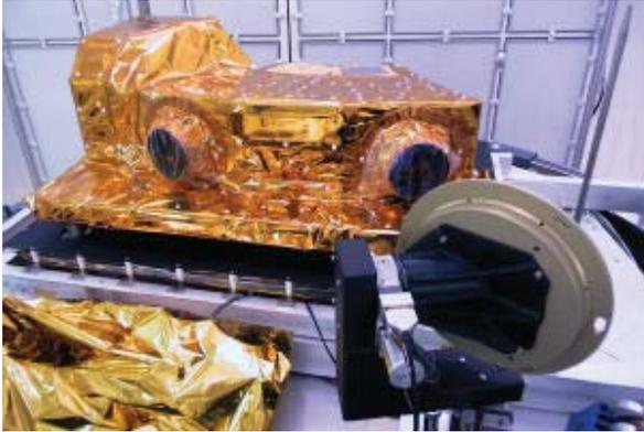
Fig.7: HRS in vacuum chamber during TB/TV tests
