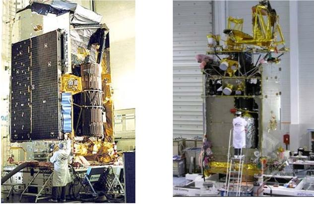
Fig. 1. Picture of Inmarsat 4 & Intelsat X satellite based on the Eurostar 3000 platform
