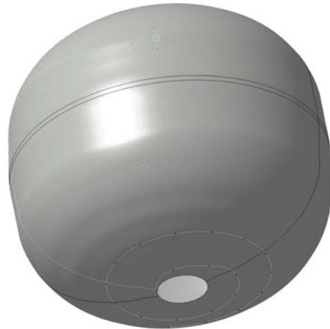
Fig. 8. Spiral mounting of the external FO temperature sensor grid
