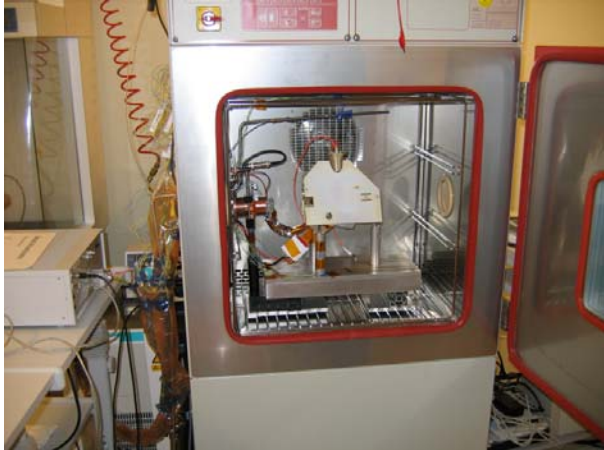
Fig. 9. Test setup in dry-nitrogen flushed climate chamber at TNO Science & Industry in Delft.
