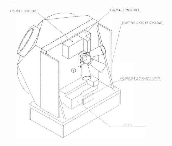
Figure 3/1: Typical instrument configuration
