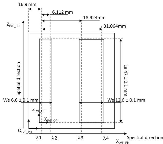
Figure 3. LVF design: HR1W and HR2W dimensioning
