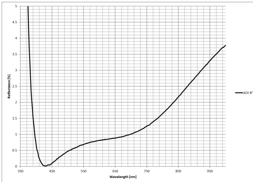
Figure 10. Measured reflectance of black coating at AOI 8°.
