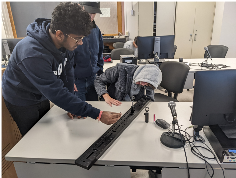
Figure 2. Students assemble a Galilean telescope on an optics rail
