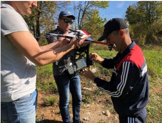
(a) Manual adjustment of the camera line of sight
