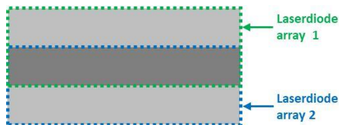
Figure 15. Sketch of acquired areas when integrating two laser diode arrays with a vertical angle shift into the transmitter assembly
