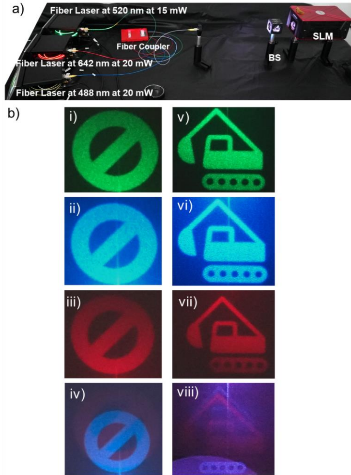
Fig. 2. Optical setup and calibration results. (a) Optical system showing a 4K SLM, RGB fiber lasers (488 nm at 20 mW), (520 nm at 15 mW), (642 nm at 20 mW), a combiner, and a beam splitter (BS). (b) Resolution targets: street sign, and construction sign to illustrate the independently controlled fiber laser sources and their alignment in full-color.
