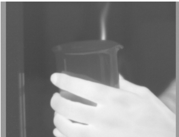
(c) Lighter behind silica glass taken by LWIR imager.
