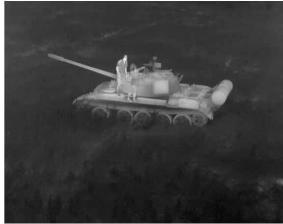
Figure 4: Instrumenting a target to measure its temperature at several locations for post-trial modelling and analysis
