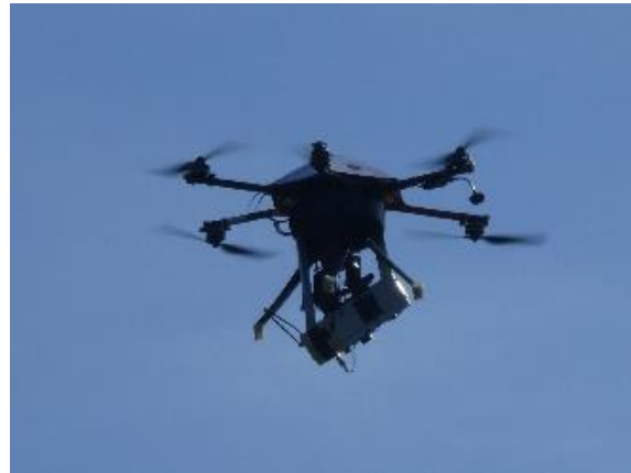
(b) Use of a 6-rotor drone for lifting a bespoke imaging and data recording system
