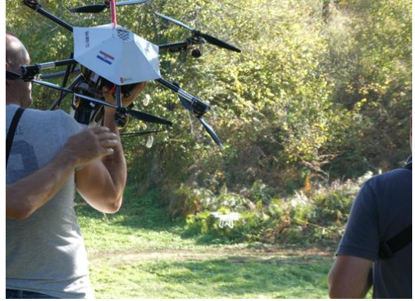
(b) Modified commercial drone (6 rotors)
