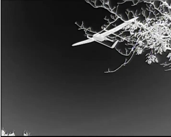
(a) Fixed-wing drone at a range of 120m
