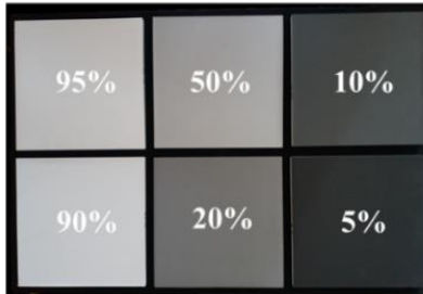
Figure 8. Diffuse reflectance targets with nominal reflectance values used for calibration
