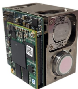
Figure 8: Photo of an eSWIR 640x512 10µm pitch module with image processing unit.
