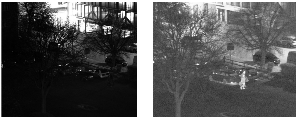
Figure 2: Detection of thermal and reflected radiation with an eSWIR 640x512 10 \mu m pitch image sensor (right) compared to a conventional visible camera (left) in a low light condition.
