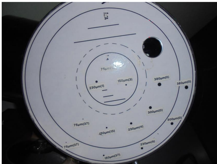
Figure 5: Example of spot defect panel used in visual inspection
