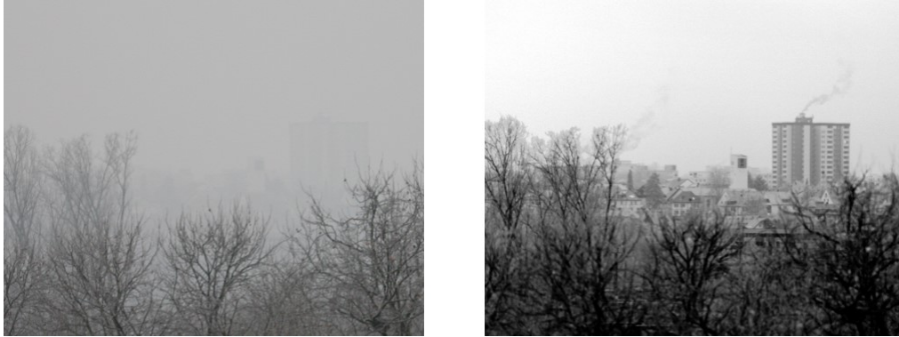
Figure 4: Comparison of images with a visible imager (left) and eSWIR 640x512 10µm pitch F/1.6 imager (right) at foggy weather condition.
