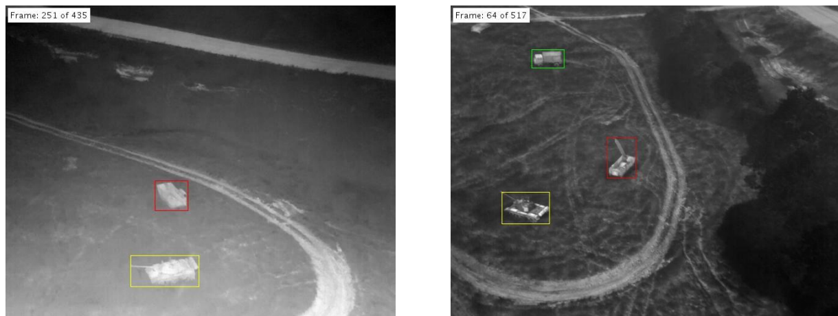
Figure 10: Annotation of multiple targets based on the use of multiple evolving template correlation.
