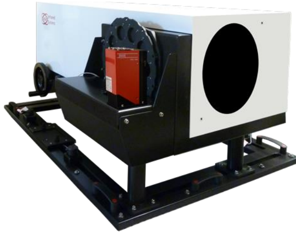
Figure 1: IRCOL Optical Test Bench
