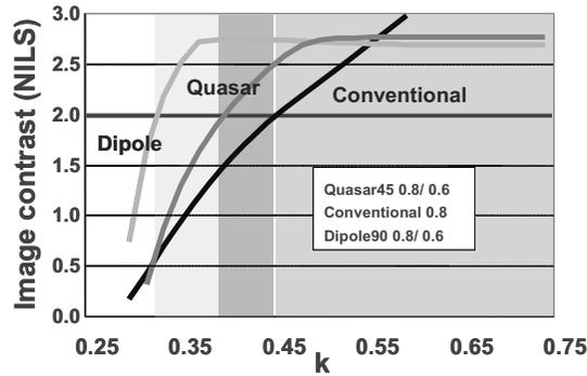
Figure 14. Image contrast as function of the k1-factor, using a 0.32NA lens.
