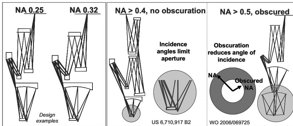
Figure 15. Possible optics design roadmap down to 11nm resolution with >0.4NA optics. All four diagrams are design examples.
