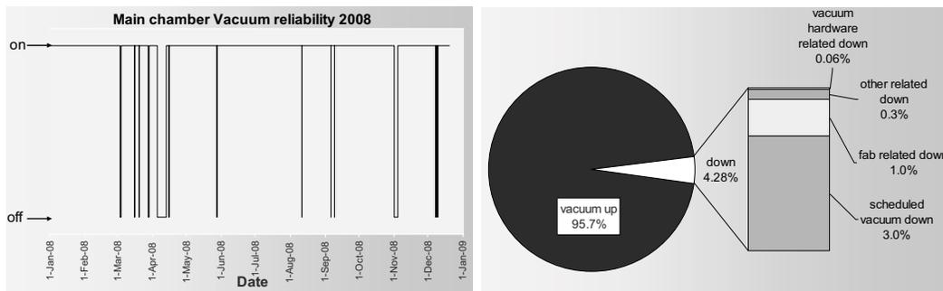
Figure 6. Vacuum reliability of the ADTs is high; the uptime of the main chamber (including optics and stages) exceeds 95%, measured over a 49-week period (total: 8232 hrs).
