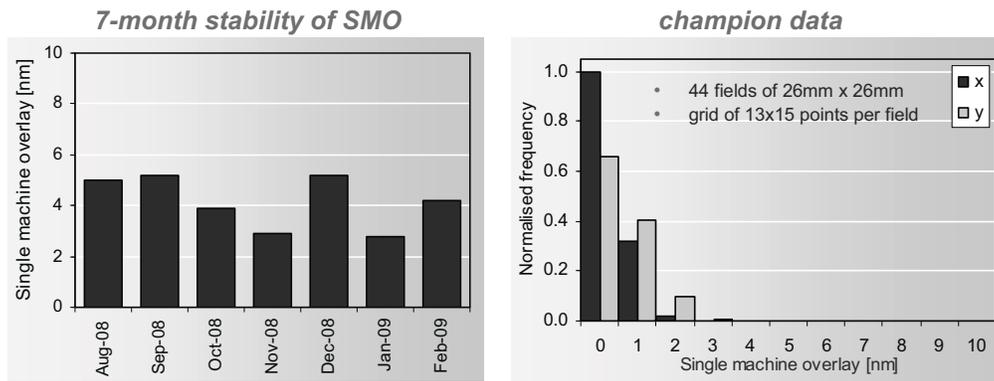
Figure 5. ADT single-machine overlay stability (left) and histogram of champion data (right).
