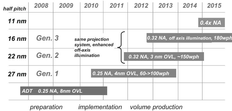
Figure 1. ASML’s NXE platform development roadmap for EUVL.
