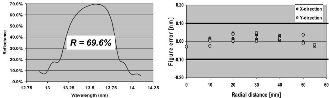
Figure 17. Left: mirror coating development for NXE has yielded >69% peak reflectivity. Right: added figure error due to the coating process for various lateral positions on the mirror.
