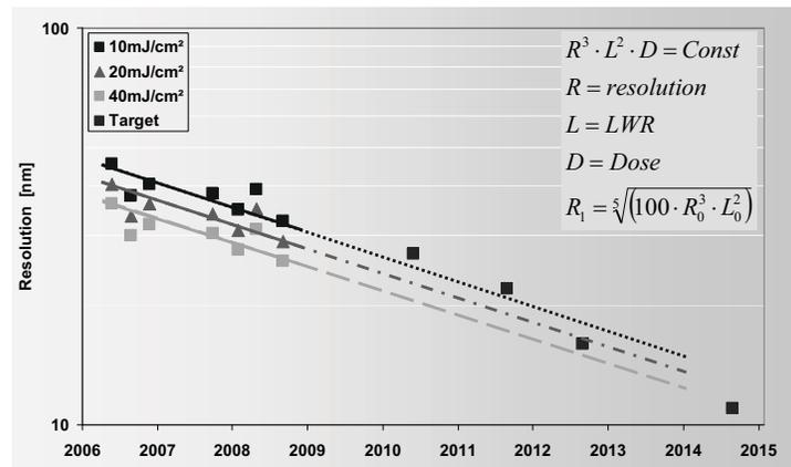
Figure 25. Resolution progress as a function of dose. All data scaled to 10% LWR.
