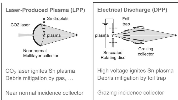
Figure 19. Key elements of sources for high volume manufacturing: LPP (left) and DPP (right).
