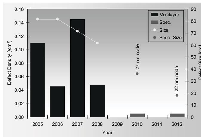
Figure 23. Progress in defect density reduction together with improvements in metrology/inspection size.
