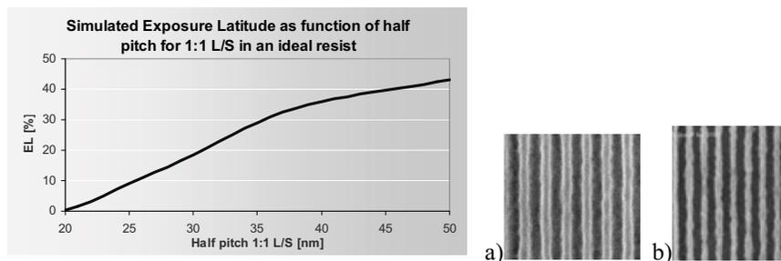
Figure 7. Left: Simulated exposure latitude as function of half pitch in an ideal resist. Right: a) 28nm<sup>[13]</sup>; and b) 26nm<sup>[15]</sup> 1:1 L/S imaging demonstrated on ADT.
