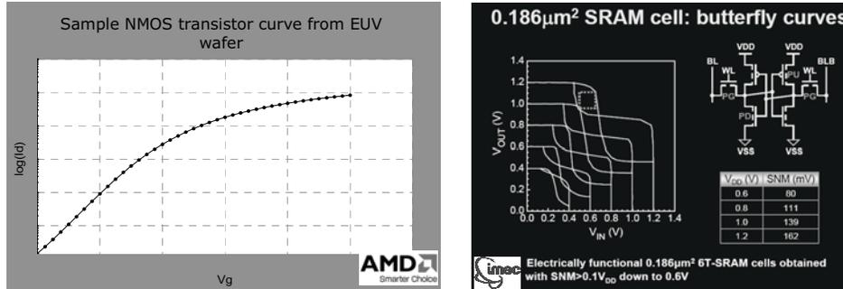
Figure 13. Left: electrically functioning transistor of which the first metal level was exposed on ADT<sup>[1]</sup>. Right: electrically functional 0.186 µm<sup>2</sup> 6T-SRAM cell, of which the contact hole layer was exposed on ADT<sup>[3]</sup>.
