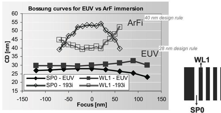
Figure 11. Bossung curves for 28nm WL1 and SP0 with EUV (NA=0.25,  $\sigma=0.5$ ) compared to 40nm WL1 and 60nm SP0 with ArF immersion (NA=1.35,  $\sigma=0.82/0.97$  dipole-X with 35° opening angle, Y-polarized)..
