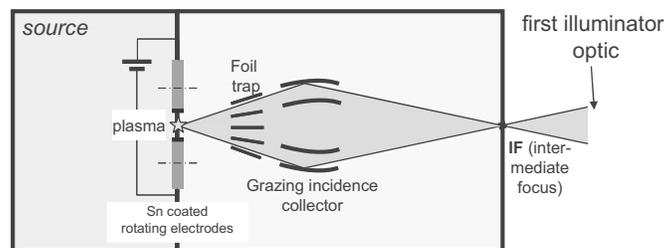
Figure 2. Schematic overview of the ADT Sn source.
