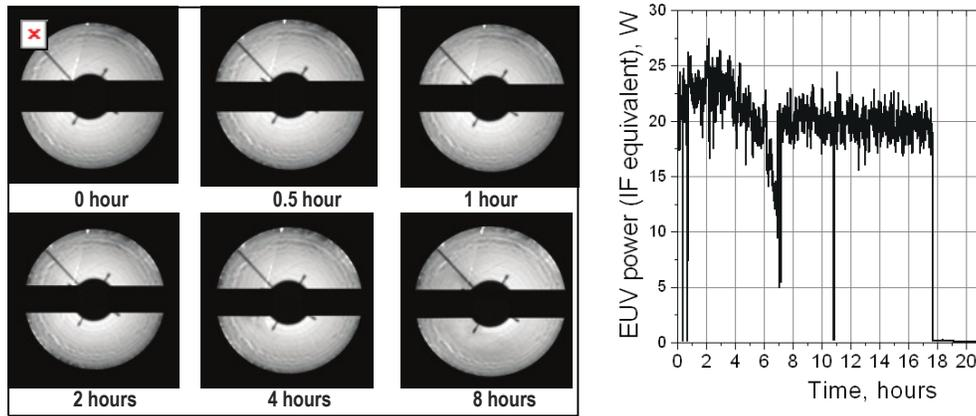
Figure 20. Left: 8hr endurance test of Cymer LPP source using fluorescent screen at the output of the source to evaluate the far-field distribution: no degradation of the images is visible, indicating that debris mitigation is functioning well. Right: 18hr source endurance test without a collector present – calculated (using a 5sr collector with 50% average reflectivity and 90% source module transmission) to have >20W in-band EUV power as output<sup>[18]</sup>.
