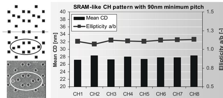
Figure 12. Left: SRAM CH pattern on our test mask and CD-SEM picture of the CHs in best focus. Process windows were measured for the 8 contacts in the encircled area. Right: Measured mean CD and ellipticity of the 8 evaluated CHs.
