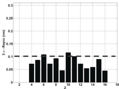
Figure 18. Aberration reproducibility versus Zernike number at the Zeiss actinic metrology test stand. Dotted line represents the requirement.
