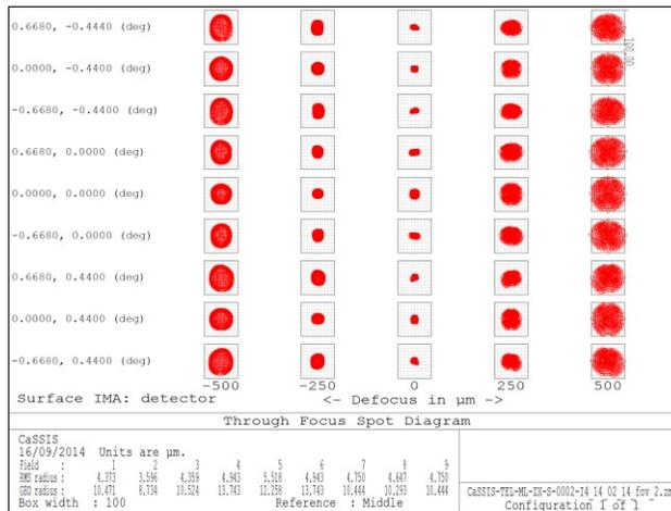
**Fig. 8** Simulated Through focus  $\pm 250$  micron at 632 nm on detector image wrt the best focus position. (via Zemax code) and the obtained RMS spot diagrams over the full CaSSIS FoV ( $1.336^\circ \times 0.887^\circ$ ) corresponding to a 20.48 mm x 13.56 mm area on the image plane of the detector. The focused spot is collected in 2x2 pixel (20 micron x 20 micron)
