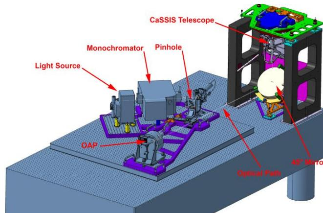
**Fig. 9** OGSE used to integrate the detector and to test the optical performances of CaSSIS. The collimated beam obtained with an 147 mm-diameter Off Axis Parabola (OAP) and a 10 μm pinhole and illuminated with either white (Quartz Tungsten Halogen) or monochromatic (10 nm FWHM bandpass) light. The CaSSIS telescope optical axis vertical via the 45 deg mirror to mitigate the effects of Earth gravity.
