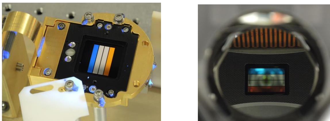
**Fig 4** Picture of the filter assembly integrated on the FPA. The FPA was illuminated by UV light to check for contamination by dust. The filter on the left of the picture is PAN, reflecting blue light and the filter on the right is BLU reflecting red and orange light. In between, the RED and NIR filters both reflect all visible light and appear like mirrors. In right side how the filters of the FPA appear through the Entrance pupil of the telescope
