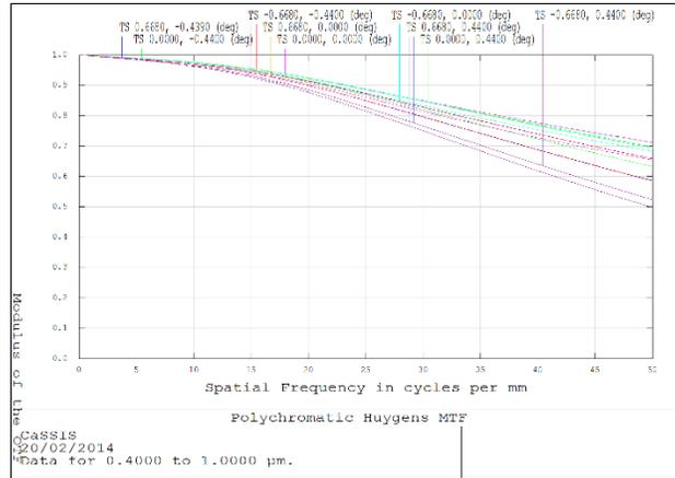
**Fig. 7** Simulated (Zemax code) polychromatic MTF (range 400-1000nm) over the full CaSSIS FoV ( $1.336^\circ \times 0.887^\circ$ ) corresponding to a 20.48 mm x 13.56 mm area on the image plane of the detector.
