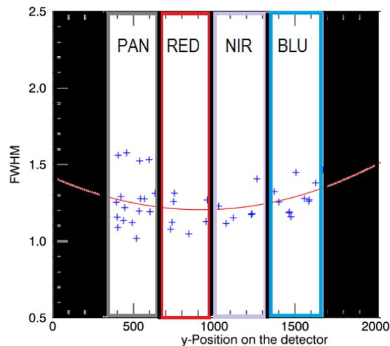
**Fig. 11** The image shows the average FWHM of the PSF as a function of the y-axis (along track) position on the detector. The filters are PAN, RED, NIR and BLU from left to right. The FWHM PSF in the different filters band is confirmed as predicted.
