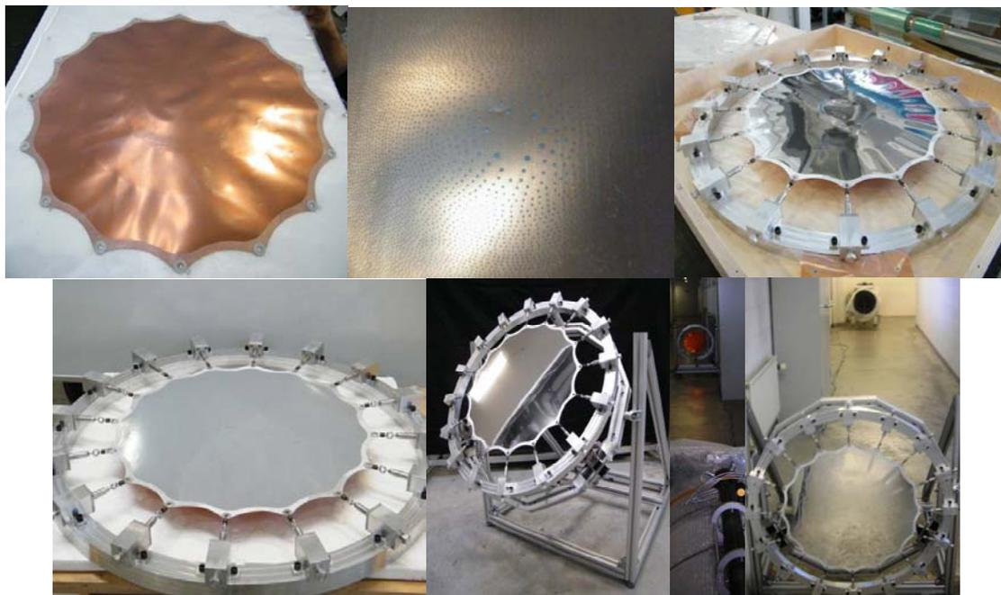
**Fig.10.** From top left to bottom right: (a) Photon-sieve after hole drilling, (b) details of the drilled holes, (c) un-stretched photon-sieve, (d) stretched photon-sieve, (e) mounted in support, and during optical test in front of a 300 mm optical collimator in a 40 m corridor.
