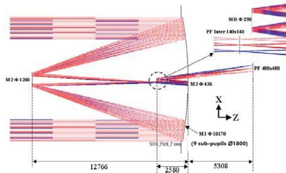
Fig. 7 Fizeau optical configuration (de-centred pupil) (lengths in mm)
