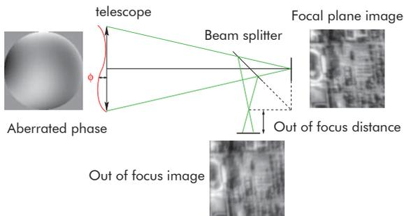
Fig. 9 Phase diversity implementation principle
