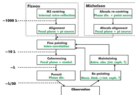
Fig. 8 Fizeau and Michelson interferometers co-phasing chronogram
