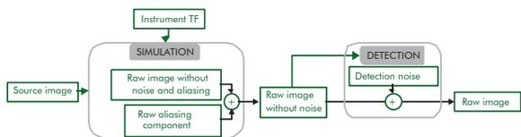
Fig. 2 Image chain simulation
