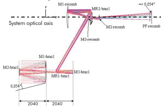
Fig. 6 One arm of the Michelson interferometer (lengths in mm)
