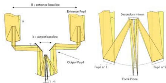
Fig. 1 Michelson (left) and Fizeau (right) interferometers
