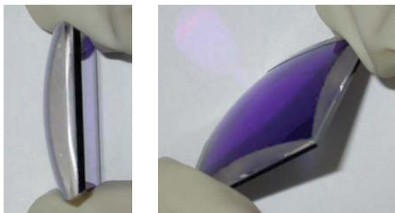
Fig. 7. Sections of Fused Silica filter lens realised.
