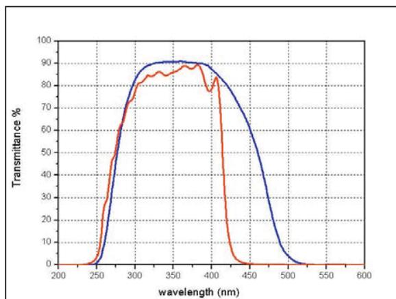
Fig. 1. Transmittance of 1mm of BG3 filter (blue line) in comparison with the transmittance of the BG3 filter covered with the realised multi-layer (red line).
