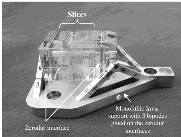
Figure 4: image of a block of slicers
