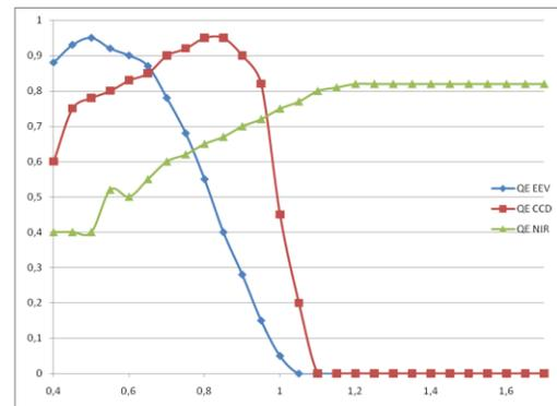
Figure 6: QE of the different detector candidates
