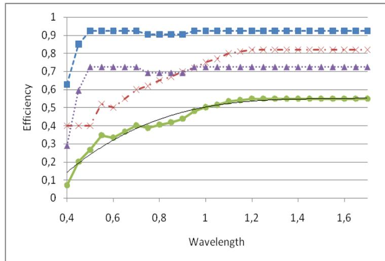
Figure 8: instrument efficiency estimation (square: telescope throughput; triangle: spectrograph throughput; crosses HgCdTe QE; round overall efficiency)
