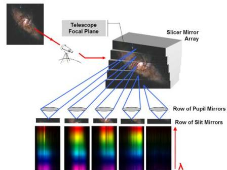
Figure 3: Image slicer principle
