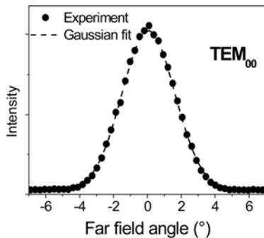
Figure 5: Transverse beam far field distribution at the output (circular symmetry), close to diffraction limit.
