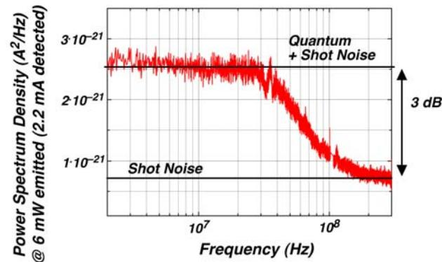
Figure 12: Intensity noise spectrum at the quantum limit.
