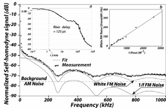
Figure 13 : Fitted and measured self-homodyne signal @  $\tau=5\mu$ s. - (inset a) : Self-homodyne  $\tau=125\mu$ s - (inset b) : White FM noise linewidth versus  $1/P_{out}$ .
