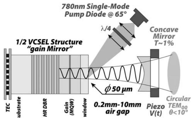
Figure 1: Single frequency Diode-pumped VeCSEL device principle and experimental setup.
