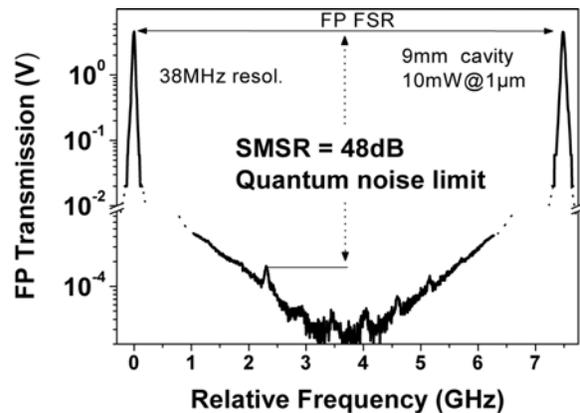
Figure 7 : SMSR Measurement obtained with a 38 MHz Confocal Fabry-Perot Interferometer.
