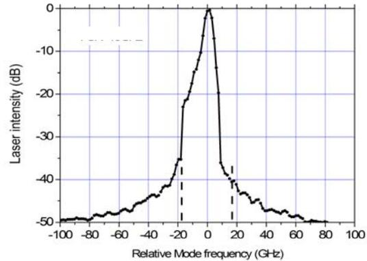
Figure 6 : Experimental laser spectrum showing single frequency operation (9mm long cavity, FSR≈17GHz).
