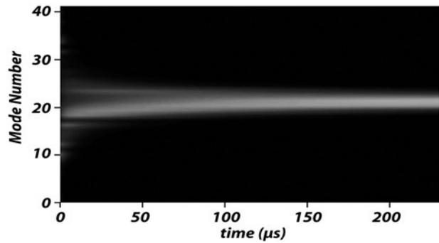
Figure 9 : Simulated VECSEL transient after start-up for an ideal homogeneous laser dynamics (electric field amplitude) without non-linear mode coupling.
