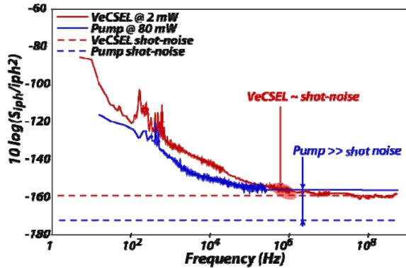
Figure 11 : Pump & VECSEL RIN versus frequency.
