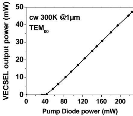
Figure 4: Continuous-wave output power at 300K for a VECSEL emitting at 1µm, pumped by a low power diode.
