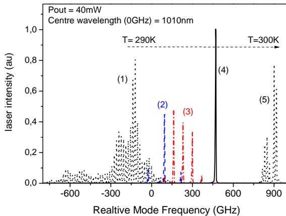
Figure 8 : Steady state Laser spectra taken at different temperatures, showing single mode stable operation at a wavelength  $\sim 1010\text{nm}$  where the  $1/2$ -VCSEL structure phase dispersion is close to zero. ( $9\text{mm}$  cavity length).
