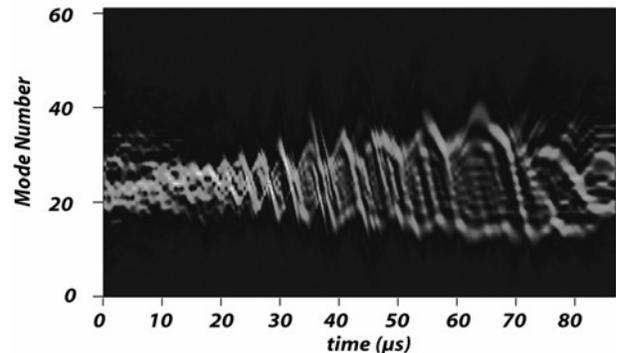
Figure 10: Simulated VECSEL transient non-linear dynamics (electric field amplitude) after start-up, for a relatively strong cavity dispersion  $\sim 10^4\text{ s}^{-1}$ .
