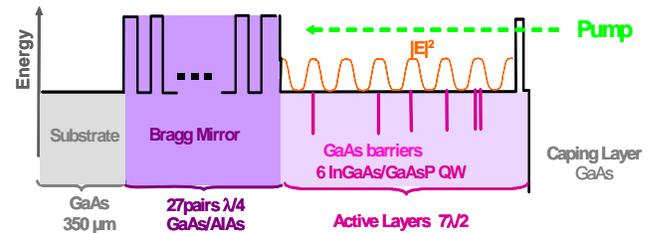
Figure 2: Typical  $\frac{1}{2}$ -VCSEL structure design grown by MOCVD exploiting GaAs based materials.
