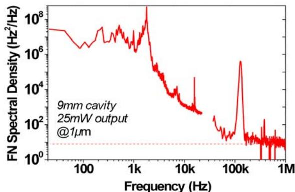
Figure 14: Low to medium frequencies FM noise spectrum: technical noise before 200 kHz and  $10 \text{ Hz}^2/\text{Hz}$  white noise limit close to the fundamental limit.
