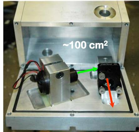
Figure 3: Laboratory low noise diode-pumped VeCSEL prototype.
