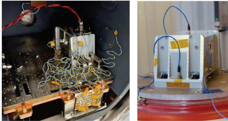
Figure 6. Environmental testing: MOONRISE EM in thermal vacuum chamber (left) and on vibration table (right).
