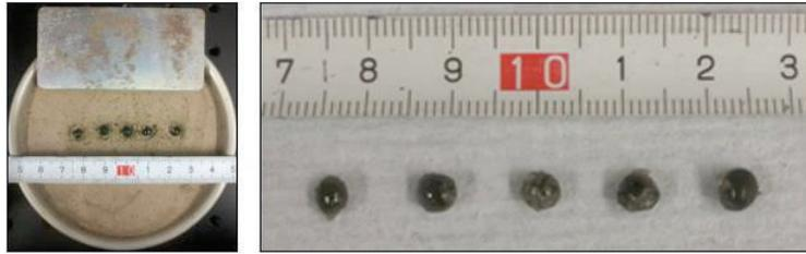
Figure 2. Laser melted regolith simulant spheres.
