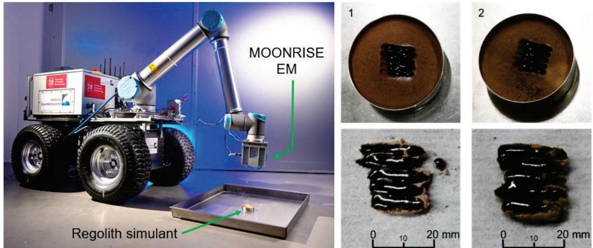
Figure 9. Typical samples of molten 2D-regolith structures (right) generated by attaching the MOONRISE EM to a robotic arm (left).
