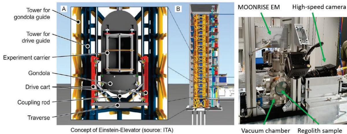
Figure 7. Schematic drawing of the Einstein-Elevator (left) and laser melting experiment prepared for the experiment carrier (right).
