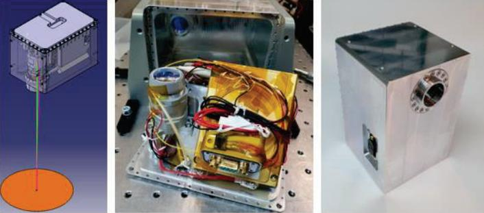
Figure 4. MOONRISE EM (from left to right): Major specification table, CAD model with laser beam, open EM, hermetically sealed EM package.
