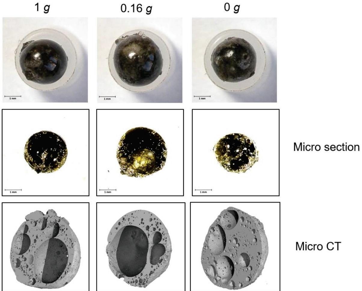
Figure 8. Typical samples of molten regolith, produced at 1 g (left column), at 0.16 g (middle) and at 0 g (right) gravity condition. The second row shows micro sections and the third row micro CT data of the processed regolith samples.
