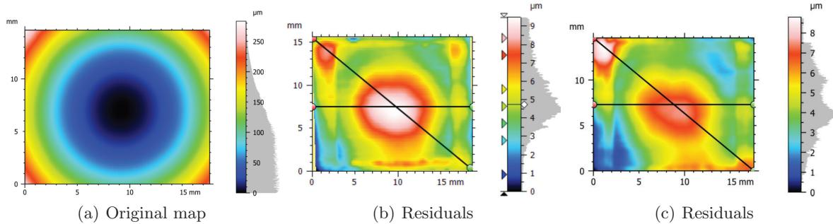
Figure 4. Surface map of a CMOS sensor curved with a radius of 250mm. a) Original Map, b) Residuals to the theoretical shape after curving, c) Residuals to the theoretical shape after curving and HTSL test
