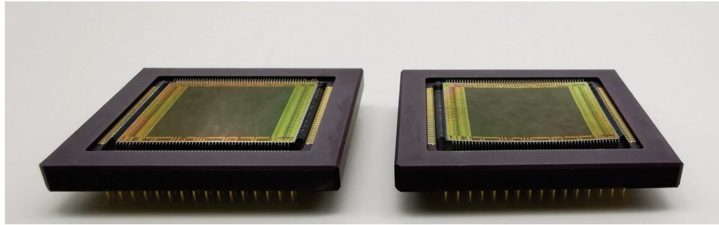
Figure 3. Pictures of packaged flat image sensor (left) and a curved image sensor(right)
