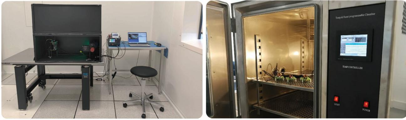
(a) EMVA 1288 electro-optical test bed
