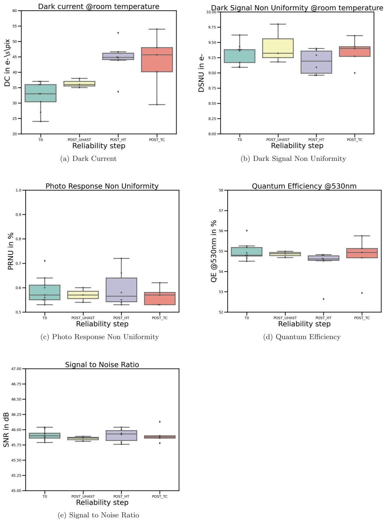
Figure 6. Electro-Optical performance after reliability tests
