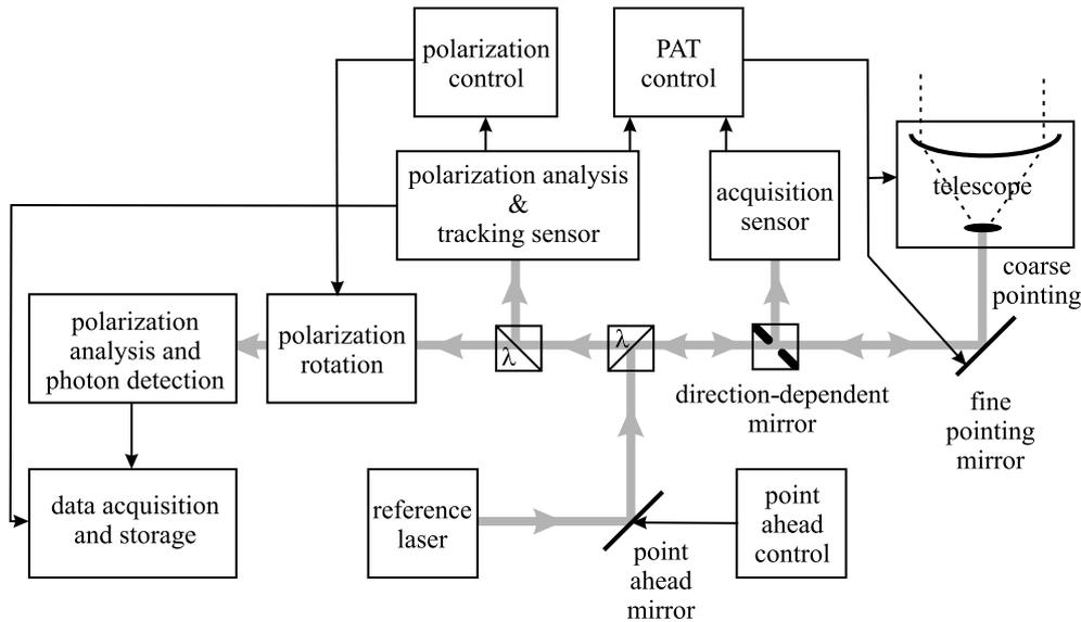
**Figure 6.** Block diagram of the receiver terminal.
