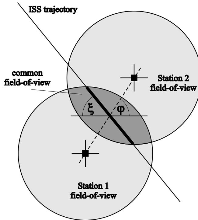
**Figure 9.** Trajectory of ISS over the field-of-view of two ground stations (the angles  $\varphi$  and  $\xi$  are measured with respect to a line parallel to the equator).
