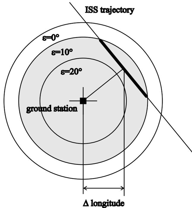
**Figure 7.** Trajectory of ISS over the field-of-view of a ground station. The possible duration of communication depends on the minimum elevation angle  $\varepsilon$  and the longitudinal shift ( $\Delta$  longitude) between the ground station and the space station in its zenith.
