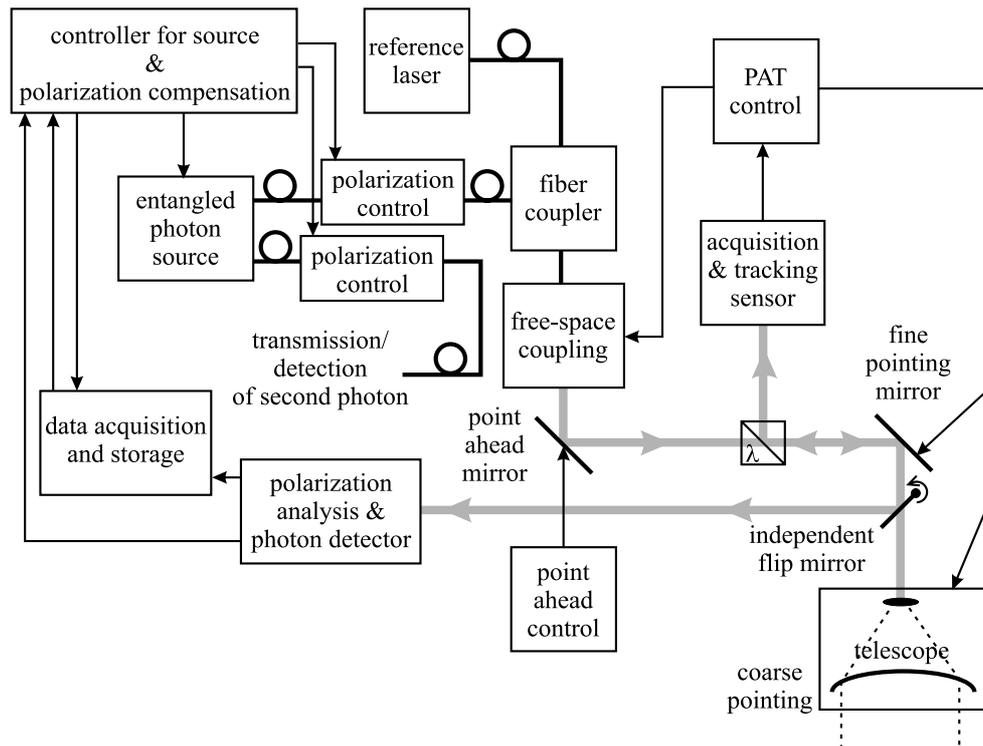
**Figure 5.** Block diagram of the transmitter terminal.
