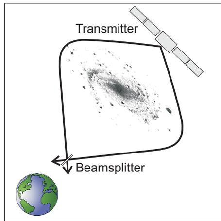
**Figure 3.** Wheeler's delayed choice experiment: the photons coming from a far source are deflected by a strong gravitational lens and brought together again to be either detected immediately or after overlapping on a beam-splitter.
