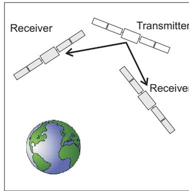
**Figure 1.** In this scheme all three terminals (one transmitter, two receivers) are placed on satellites. This provides maximal flexibility for a wide range of experiments over long distances without any losses due to atmospheric effects.
