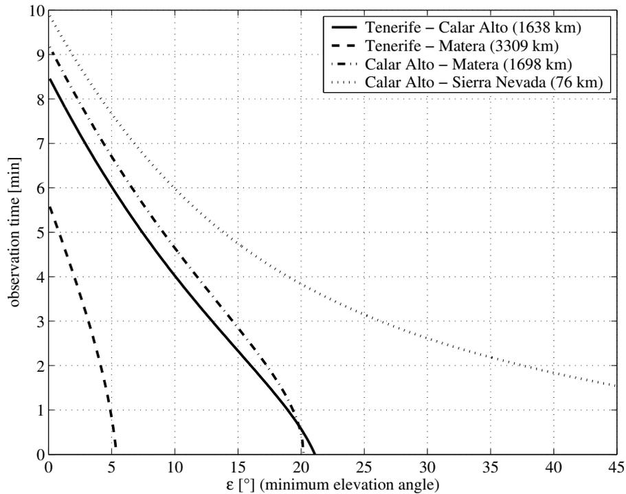
**Figure 10.** Maximum duration of simultaneous communication between ISS and two ground stations as a function of the elevation angle. (The distance cited in the insert is that between the stations.)
