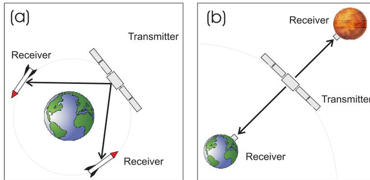
**Figure 2.** (a) Scenario in which two astronauts and the source of entangled photon pairs are separately orbiting Earth. Due to their different propagation velocities there will naturally be periods of time where the necessary distances are reached. (b) Scenario for a Bell experiment with one astronaut on (or near) Earth, one on (or on the way to) Mars and the source of the entangled photon pairs on an orbit in between.
