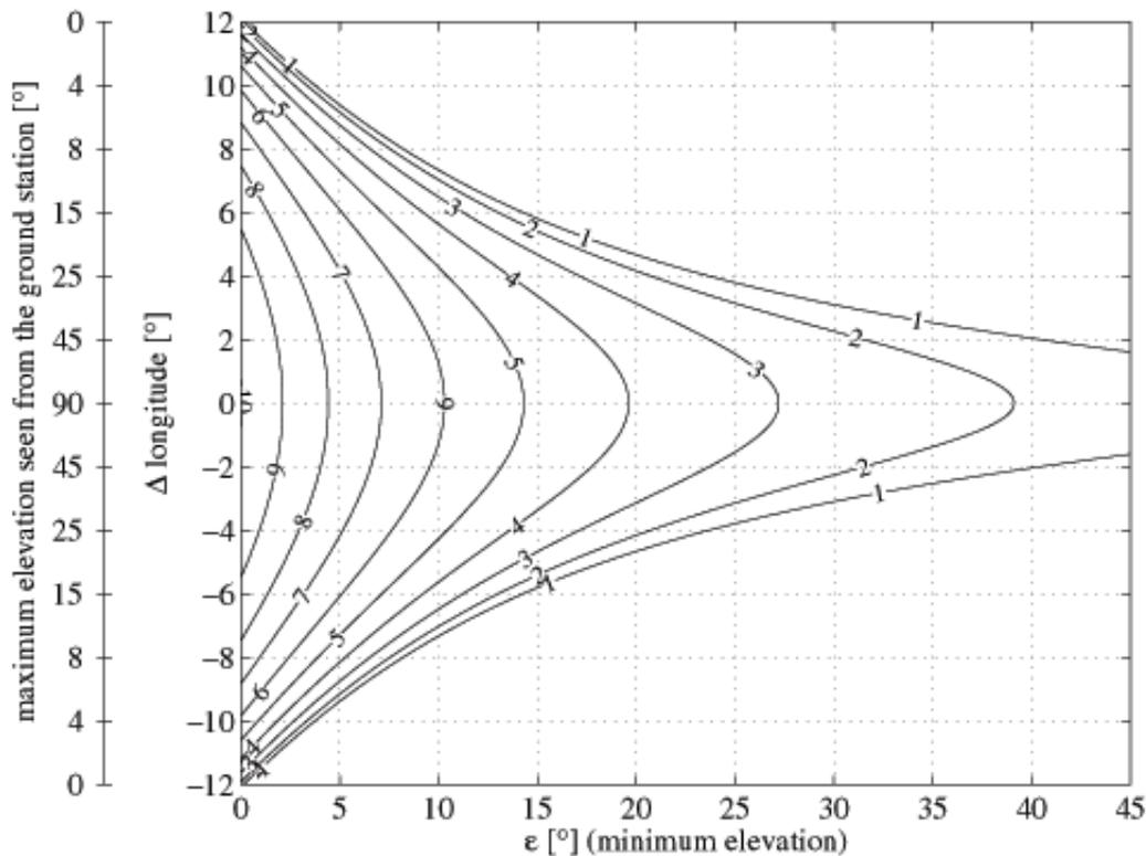
**Figure 8.** Maximum duration of communication between ISS and the OGS (given in minutes by the numbers inserted along the lines) as a function of the elevation angle and the difference in longitude of the ground station and the satellite when in zenith.
