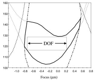
*printed with a specified depth of focus* [4]. The specification for DOF is governed by the magnitude of the process errors present in the manufacturing process, while the DOF itself is used as a proxy for the full range of process latitudes that govern the resulting CD control.
