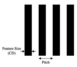
determines the characteristics and performance of an individual transistor, and has the greatest impact on chip speed and power consumption. Obviously both are very important.
