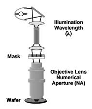
Pitch resolution is the classical resolution discussed in most optics textbooks and courses. It is governed by the wavelength of the light used to form the images and the numerical aperture of the imaging lens. The classical pitch resolution is given by a version of the Rayleigh equation
