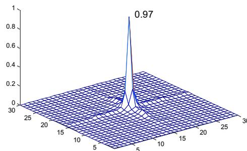
Fig. 6. Normalized output plane for the decoded signature obtained from a rotated version (80 degrees) of the ID tag (Fig. 4). Parameter  $k=0.5$  is used.
