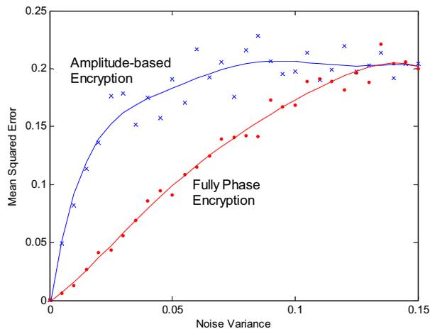
Fig. 12. Mean-squared-error for the decrypted signatures using amplitude-based encryption and fully phase encryption.
