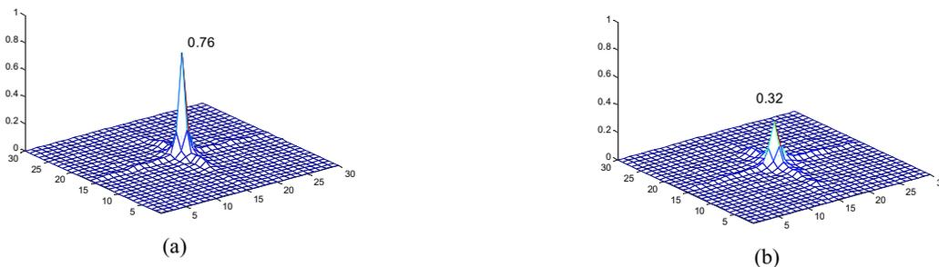
Fig. 8. Normalized output planes for the decoded signatures obtained from rotated version of the ID tag (Fig. 4). Parameter  $k=0.5$  is used. The ID tag was scaled by a factor (a) 0.2, and (b) 0.1.
