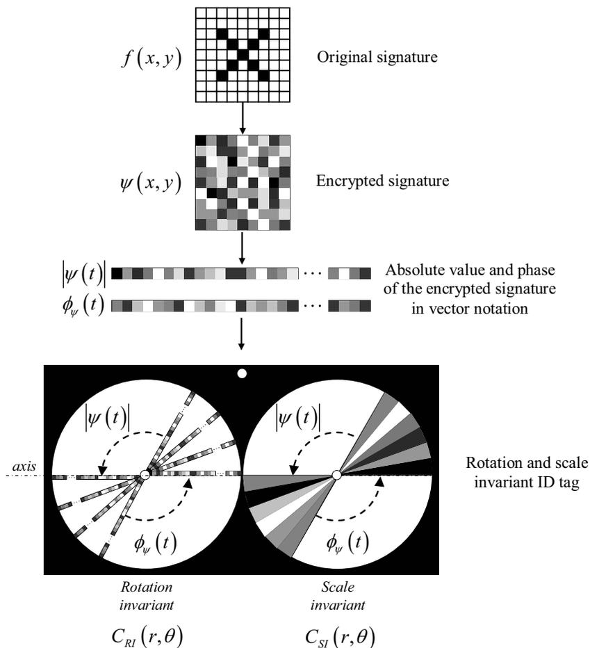
Fig. 2. Synthesis of a distortion (rotation and scale)-invariant ID tag.
