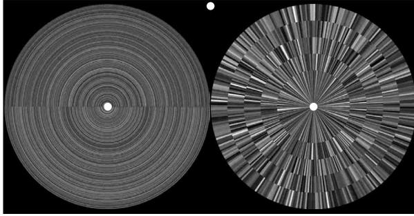
Fig. 4. Example of distortion-invariant ID tag built from an encrypted signature with a large number of pixels (Fig. 1). The information of the optical code in the scale-invariant tag (circle on the right) is distributed in concentric circles.
