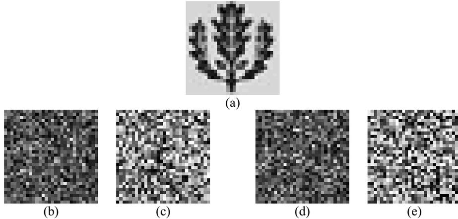
Fig. 1. (a) Signature  $f(x, y)$ ; (b) Magnitude and (c) phase of the amplitude-based encrypted signature  $\psi_A(x, y)$ ; (d) Magnitude and (e) phase of the fully phase encrypted signature  $\psi_P(x, y)$ .
