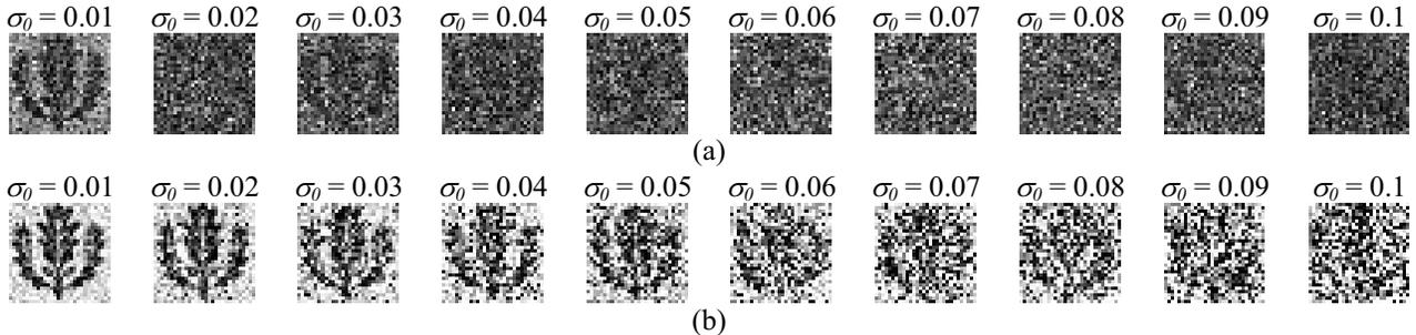
Fig. 11. Decrypted signatures for distortion-invariant codes affected by additive zero-mean Gaussian noise of different variance  $\sigma_0$ . (a) Results for the amplitude-based and (b) fully phase encryption methods.
