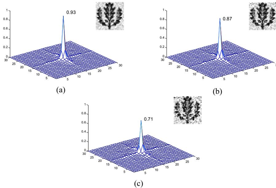
Fig. 9. Decoded signatures and correlation outputs ( $k=0.5$ ) for simultaneously rotated and scaled versions of the ID tag shown in Fig. 4. (a) Scale factor:  $\times 0.5$  and rotation angle:  $60^\circ$ ; (b) Scale factor:  $\times 0.4$  and rotation angle:  $70^\circ$ ; (c) Scale factor:  $\times 0.3$  and rotation angle:  $80^\circ$ .
