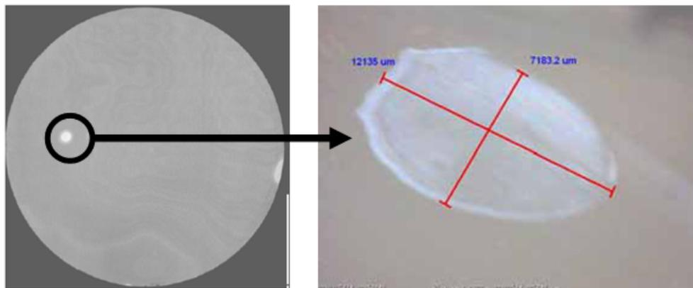
Figure 4. SAM image of bonded wafer with particle-induced void. Silicon bubble delaminated from carrier wafer following wafer thinning.
