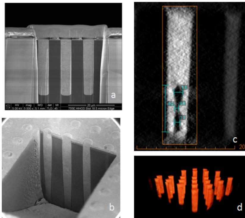
Figure 8. Destructive techniques used for TSV void detection include cross section FIB-SEM (a), whole wafer FIB-SEM (b), X-ray microscope (c) and X-ray computed tomography for 3D virtual reconstructions (d).
