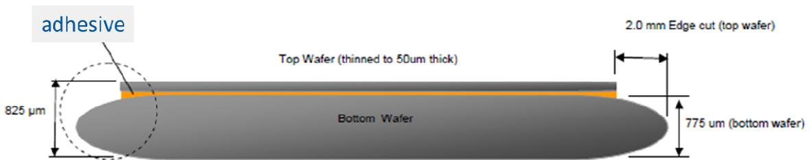
Figure 6. Edge-bevel trim to control edge chipping during wafer thinning.
