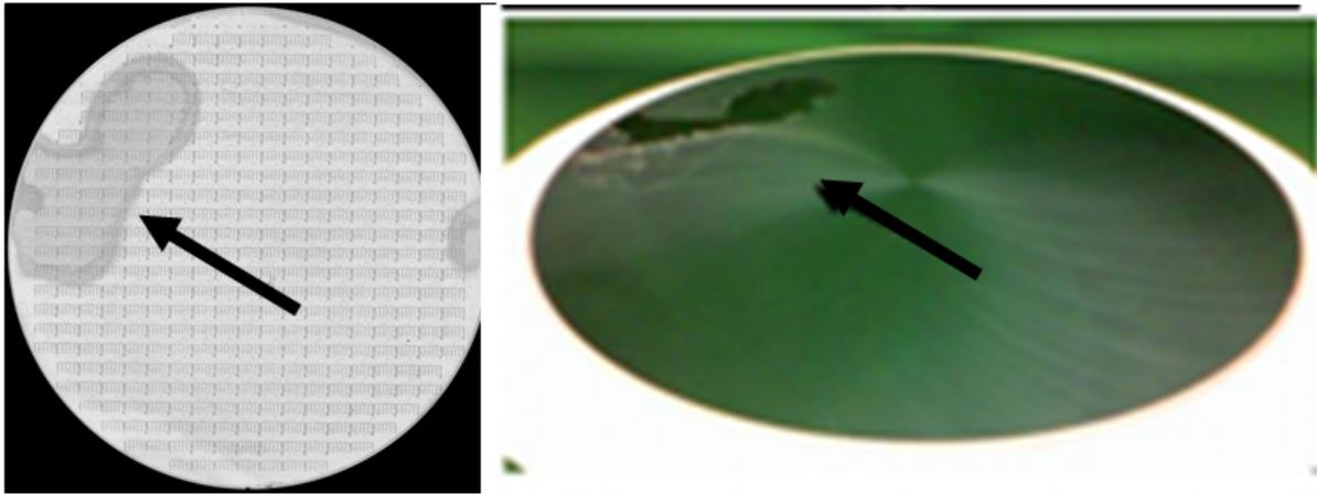
Figure 3. SAM image of bonded wafer pair on left (adhesive issue). Top wafer shredding during grinding is shown on right.
