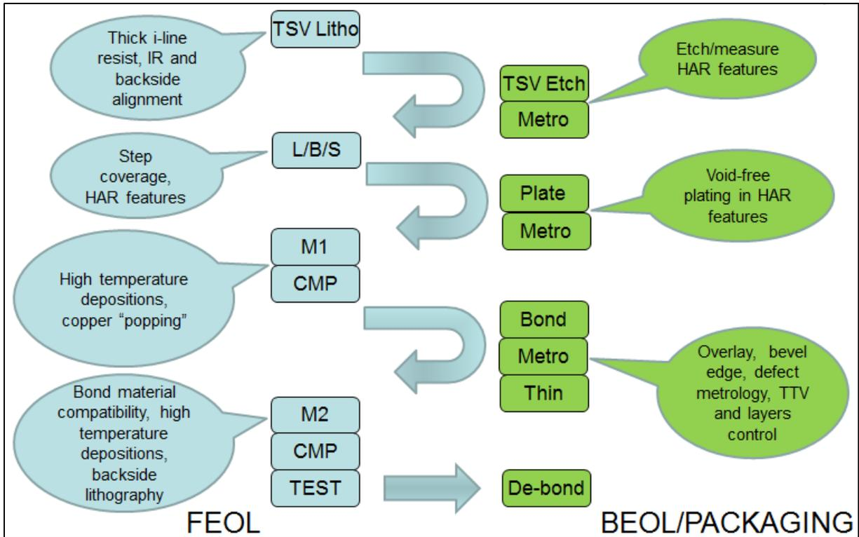
Figure 1. Process flow for via-mid TSV integration. Wafers can move from the front end-of-line (FEOL) to back end-of-line (BEOL) on TSV and traditional packaging tools and return to the FEOL for subsequent processing. Metrology and 3D integration process challenges that result are highlighted.
