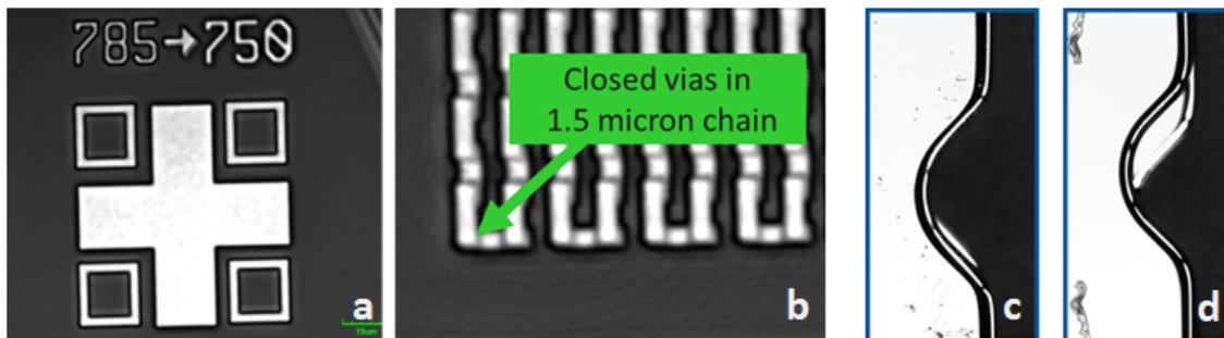
Figure 2. IR microscope image - Alignment fiducial showing good wafer-to-wafer overlay (a). IR microscope image - electrically yielding via chains resulting from good overlay (b). Visible microscope image of properly aligned bonded wafer pair notch (c). Improperly aligned bonded wafer notch can cause process tool wafer pre-aligner issues (d).
