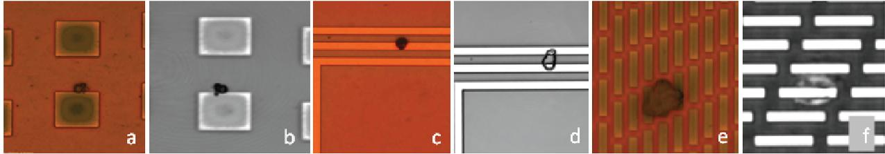
Figure 5. Defect viewed in visible light on single wafer (a), (c), (e). Same defects viewed using IR microscope at interface of a bonded wafer pair (b), (d), (e). Defect (c) modified by bonding now bridges two lines (d) at interface of bonded pair. Defect (e) is partially obscured by opaque layer (f) at interface of bonded wafer pair.
