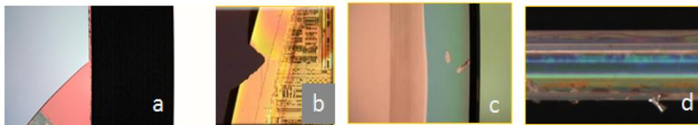
Figure 7. Delamination following wafer thinning (a), edge-bevel chip (b), edge-bevel defects (c), (d).
