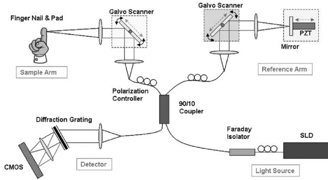
**Fig. 1** Schematic of the FD-OCT used for evaluating complex conjugate removal methods. Three dotted rectangles represent components that are used to introduce phase shifts that were tested: SLD (superluminescent diode), CMOS (complementary metal-oxide semiconductor) line detector, and PZT (piezoelectric translator).
