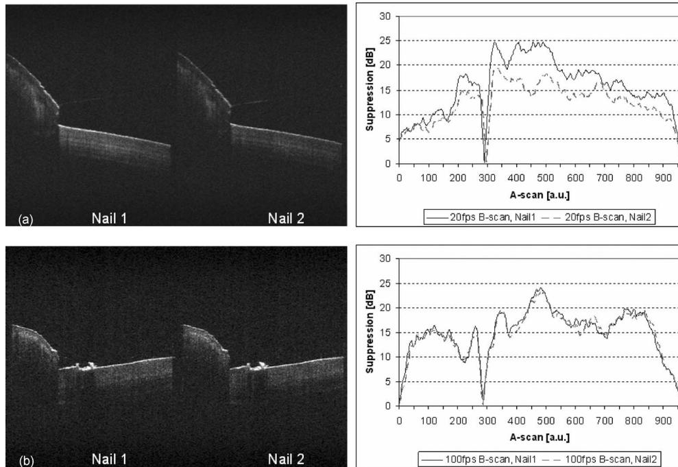
**Fig. 6** Decreasing suppression ratio by sample movement. B-scan images with the sample arm pivot offset method ( $\Delta\varphi=0.5\pi$ ) of *in vivo* human fingernail images at a stationary position Nail 1, and the sample moved Nail 2 (left), and complex conjugate suppression ratio of Nail 1 and Nail 2 (right). Fingernails at (a) 20-fps B-scan, (b) 100-fps B-scan, and the suppression ratio. The lateral scanning range of each nail image is 6 mm.
