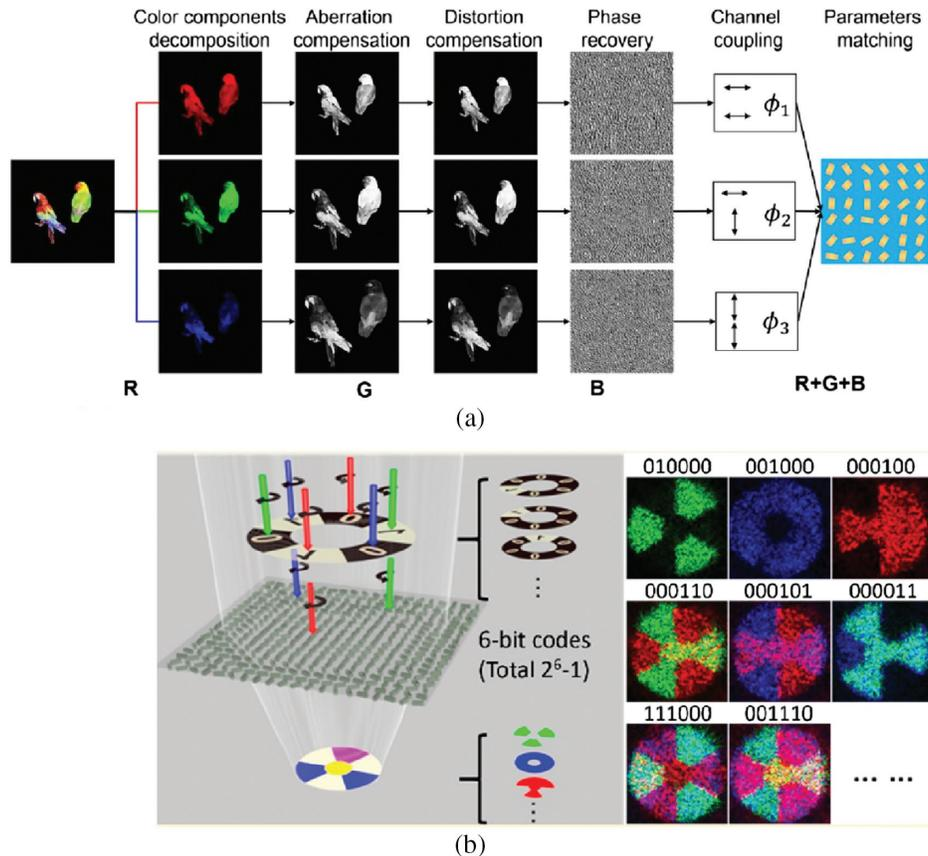
**Fig. 2** Multicolor holograms by the polarization multiplexing method. (a) Design process for the vectorial color holographic metasurface. (b) Schematic of 6-bit metasurface. Holographic images that result from the state (color and polarization) of the incident light as denoted by codes 010000, 001000, 000100, 000110, 000101, 000011, 111000, and 001110 are shown in the right panel of the image. Figures reproduced with permission from (a) Ref. 64 and (b) Ref. 75.
