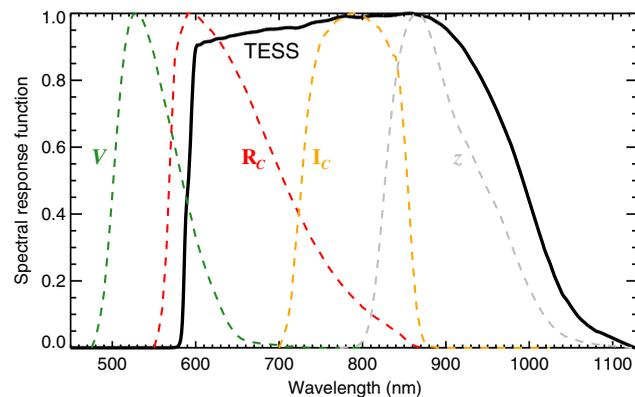
**Fig. 1** The Transiting Exoplanet Survey Satellite (TESS) spectral response function (black line), defined as the product of the long-pass filter transmission curve and the detector quantum efficiency curve. Also plotted, for comparison, are the Johnson–Cousins  $V$ ,  $R_C$ , and  $I_C$  filter curves and the Sloan Digital Sky Survey  $z$  filter curve. Each of the functions has been scaled to have a maximum value of unity.
