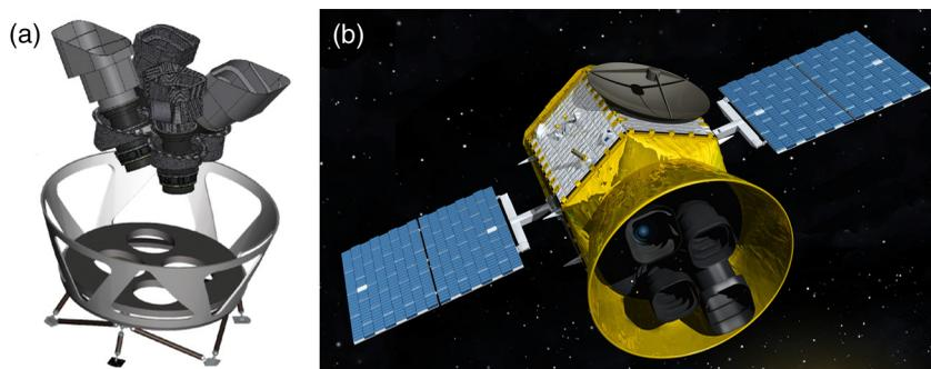
**Fig. 4** (a) Diagram illustrating the orientations of the four TESS cameras, lens hoods, and mounting platform. (b) Artist's conception of the TESS spacecraft and payload.
