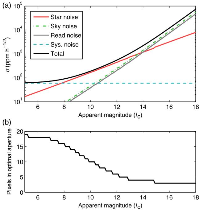
**Fig. 8** (a) Expected  $1\sigma$  photometric precision as a function of stellar apparent magnitude in the  $I_C$  band. Contributions are from photon-counting noise from the target star and background (zodiacal light and unresolved stars), detector read noise ( $10 e^-$ ), and an assumed 60 ppm of incorrigible noise on hourly timescales. (b) The number of pixels in the photometric aperture that optimizes the signal-to-noise ratio.
