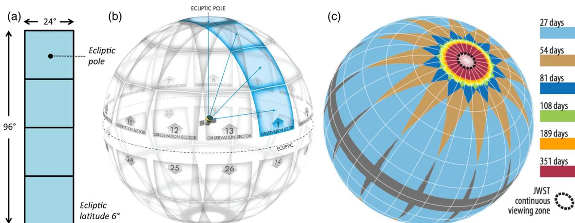
**Fig. 7** (a) The instantaneous combined field of view of the four TESS cameras. (b) Division of the celestial sphere into 26 observation sectors (13 per hemisphere). (c) Duration of observations on the celestial sphere taking into account the overlap between sectors. The dashed black circle enclosing the ecliptic pole shows the region which James Webb Space Telescope will be able to observe at any time.
