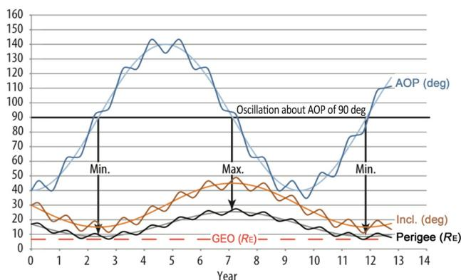
**Fig. 6** Calculated time variations in the elements of the nominal TESS mission orbit. The units of each curve are specified in the legend. AOP is the argument of perigee. GEO is the geosynchronous Earth orbit.
