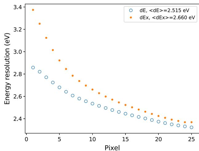
**Fig. 11** Simulation predicting the FWHM energy resolution of the  $5 \times 5$  hydra sensor with 800-nm pitch meander coils in the MMC main array in LXM. The energy resolution without errors in position correlation is dE, whereas dEx includes the effect of uncertainty in determining the x-ray absorption location in the  $5 \times 5$  hydra for an x-ray energy of 200 eV. For x-ray energies much larger than 200 eV, the energy resolution approaches dE.
