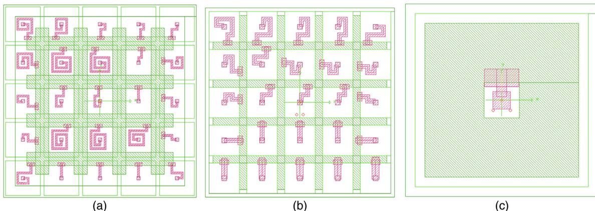
**Fig. 1** Layout of (a) main, (b) enhanced, and (c) UHR MMC sensors. The Au:Er sensor (green shaded), Au thermal links (red shaded) between sensor and x-ray absorber support stems, and Au x-ray absorbers (green open) are shown. Absorber size is 50, 25, and 50  $\mu\text{m}$ , respectively, for main, enhanced, and UHR sensors, whereas the overall hydra unit cells shown have sizes 250, 125, and 50  $\mu\text{m}$ .
