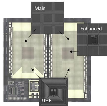
**Fig. 8** Die layout of prototype MMC LXM array. The  $22 \text{ mm} \times 22 \text{ mm}$  reticle is divided into two chips differing only in size. Insets show locations of main array, enhanced array, and UHR array pixels.
