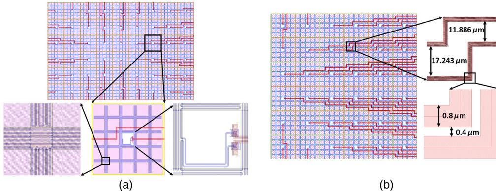
**Fig. 6** (a) LXM enhanced array sensor design with successive close-ups of one Au:Er waffle sensor, the top level Nb sensor coil that meanders to fill the area under the Au:Er waffle, and the interconnection to lower wiring layers, through near the center of the waffle, to a twin-microstrip wire pair and ground plane. (b) Details of the Nb wiring in lower level muntins, which are shielded from the main array wiring and sensors by the intervening ground planes.
