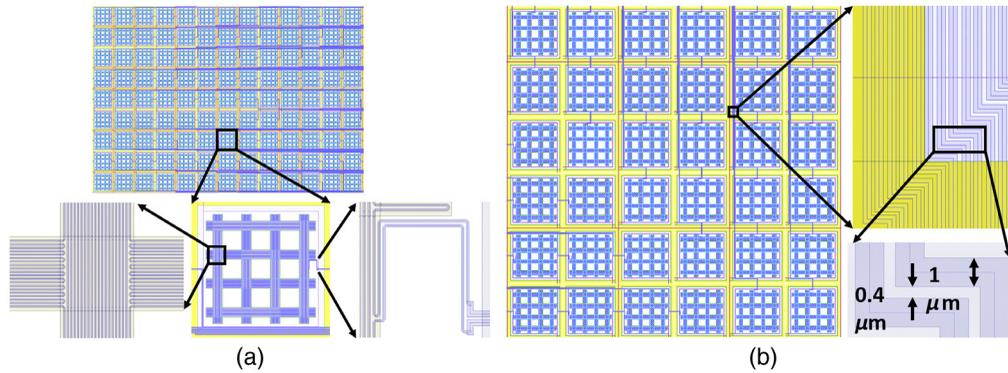
**Fig. 5** (a) LXM main array sensor design with successive close-ups of one Au:Er waffle sensor, the Nb sensor coil that meanders to fill the area under the Au:Er waffle, and the interconnection to a twin-microstrip wire pair over a Nb groundplane in an adjacent muntin. (b) Details of the Nb wiring in the muntin, which is partially covered by a Au heat sinking grid.
