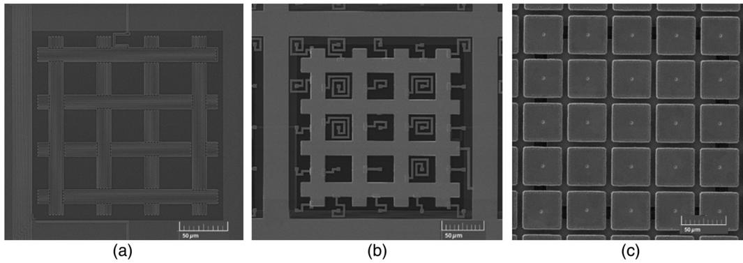
**Fig. 9** Evolution of a main array hydra sensor during fabrication. (a) Sensor meander coil laid out in a waffle shaped pattern. (b) After deposition of Au:Er, heat sinking grid and hydra thermal links. (c)  $5 \times 5$  hydra of  $2.8\text{-}\mu\text{m}$  thick electroplated Au absorbers suspended over sensor. The overall hydra size is  $250\ \mu\text{m} \times 250\ \mu\text{m}$ .
