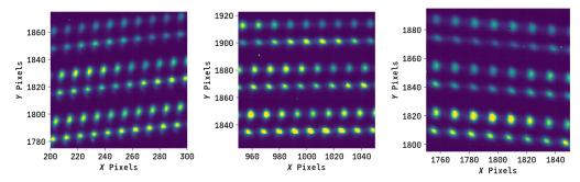
**Fig. 2** Raw PARVI frame of the LFC injected through the science (top) and calibration (bottom) fibers. We show the same three orders m = 89 to 91 across the detector (top to bottom; wavelength increases from left to right). The tilt in the PSF is different for the two fibers and changes across each order (and orders). The colormap is arbitrarily scaled for adequate contrast.
