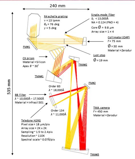
**Fig. 1** Schematic showing the layout of the cross-dispersed echelle spectrograph, which is designed to achieve  $R \sim 87,000$  to 121,000 in a compact 0.5 m  $\times$  0.25 m optical bench through the use of a SMF input from the Palomar AO system.
