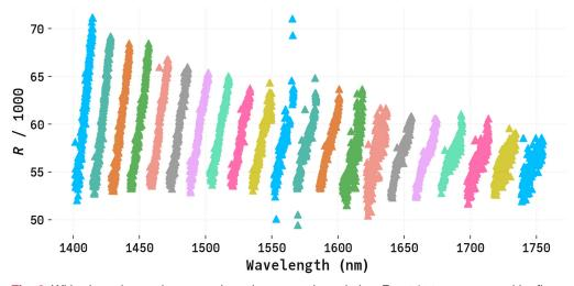
**Fig. 3** With triangular markers, we show the spectral resolution  $R = \lambda/\Delta\lambda$  as measured by fits to individual 1D LFC modes. Each like-color corresponds to a like-order (m = 85 to 105). Due to PARVI's compact construction, the effective spectral resolution of the 1D spectrum changes by  $\approx 20\%$  within an order.
