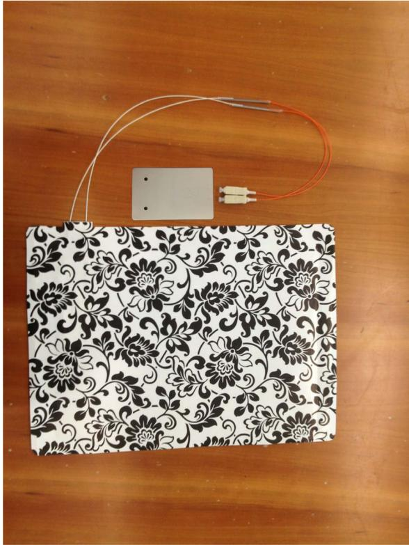
**Fig. 10** Prototype system of the microbend fiber optic sensor mat and transceiver.
