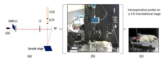
**Fig. 1** SFD-qFl setup: (a) schematic diagram showing the liquid light guide, DMD, lenses (L1, L2), mirror (M), LCTF, CCD, and the sample stage, (b) photograph of the system as well as the point probe mounted on a 3-D translation stage, and (c) close-up of a rat affixed to the stereotaxic frame with the probe positioned for point qFS measurements.
