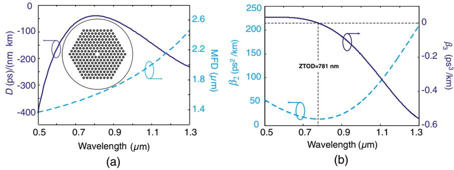
**Fig. 1** (a) Calculated dispersion profile and mode field diameter of ANDi-MOF. (b) Corresponding spectral dependencies of second- and third-order dispersion coefficients.
