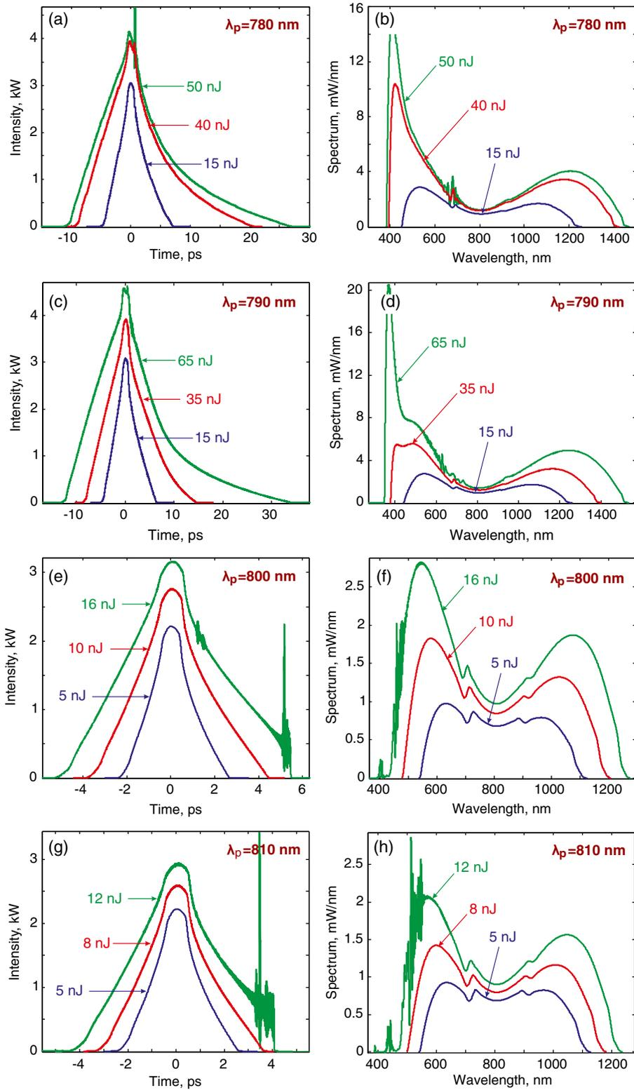
**Fig. 4** SPSC spectra (b, d, f, h) and corresponding broadened pulses (a, c, e, g) at the output of designed ANDi-MOF for different pump wavelengths and initial pulse energies. Fiber length is 10 cm.
