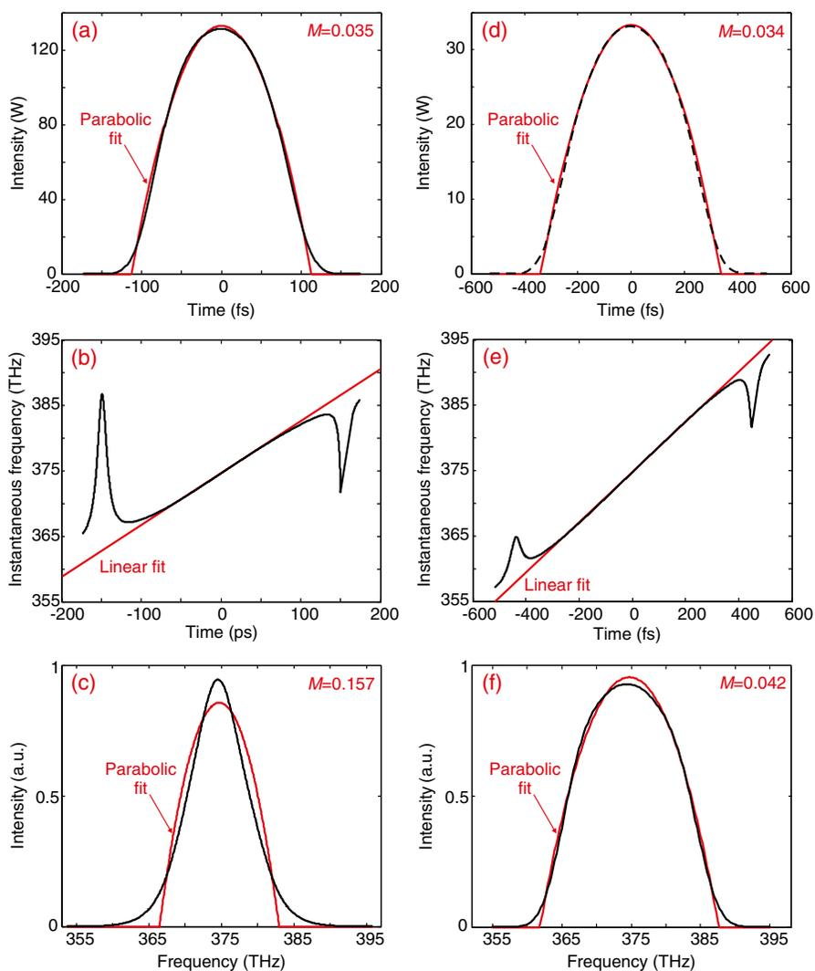
**Fig. 3** Parabolic pulses generated in ANDi-MOF. Left column (a, b, and c) shows the results (temporal intensity, chirp, spectrum) of parabolic pulses obtained from initial unchirped Gaussian pulse ( $\tau_0 = 80$  fs,  $E_0 = 20$  pJ) at fiber length of 10 cm. Right column (d, e, and f) shows the result of parabolic pulse obtained in the steady-state propagation regime from initial chirped Gaussian pulse ( $\tau_0 = 80$  fs,  $E_0 = 15$  pJ,  $C = 1.24$ ) at fiber length of 30 cm.
