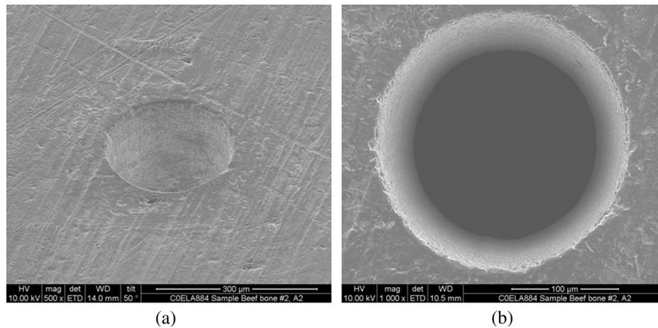
**Fig. 8** Micro-hole drilling in bovine bone using fs fiber laser: (a) SEM overview and (b) SEM top view.
