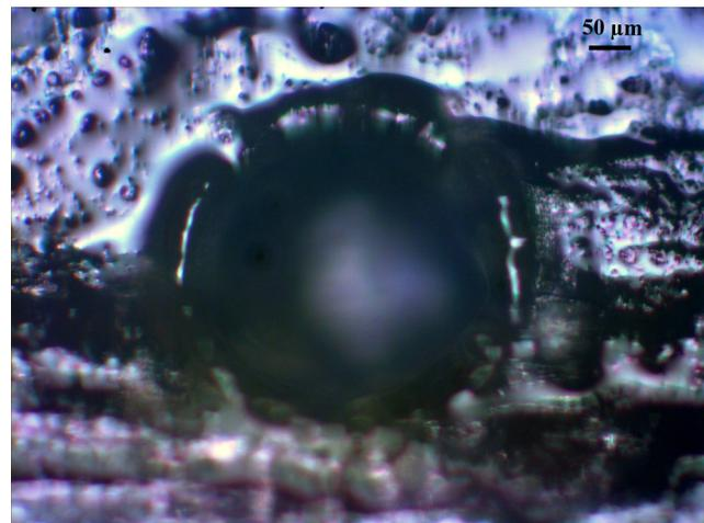
**Fig. 9** Microscope view of micro-hole drilling in bovine tendon using fs fiber laser.
