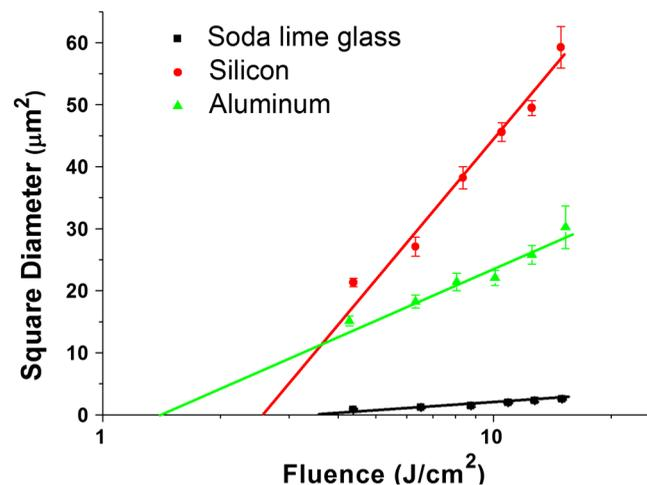
**Fig. 2** Single-shot ablation threshold measurement for different materials by using fs laser.
