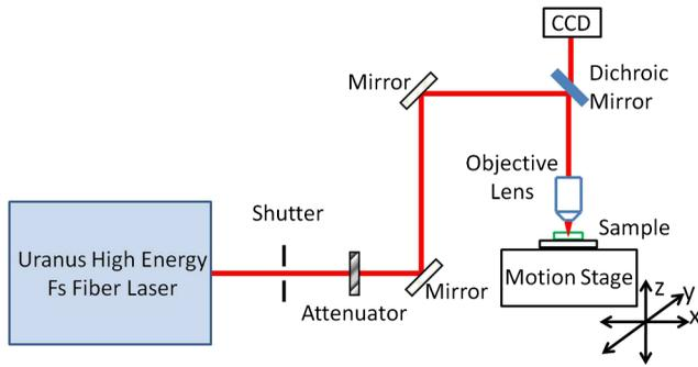
**Fig. 1** Experimental setup for fs laser micromachining using microscope objective.
