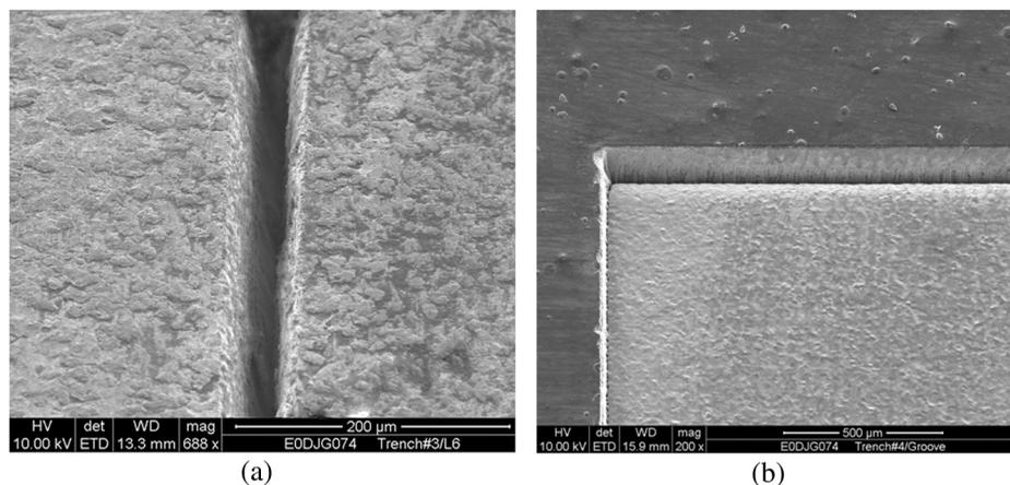
**Fig. 11** SEM view of titanium trench and micro-cavity micromachining by using fs fiber laser. (a) Trench micromachining and (b) micro-cavity micromachining.
