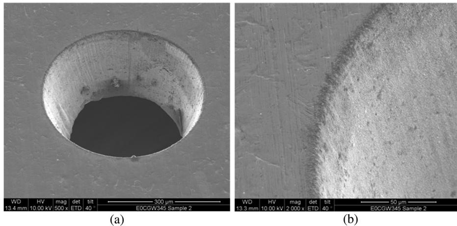
**Fig. 5** SEM view of the drilled hole in stainless steel using fs fiber laser: (a) Overview and (b) detail view of hole sidewall.
