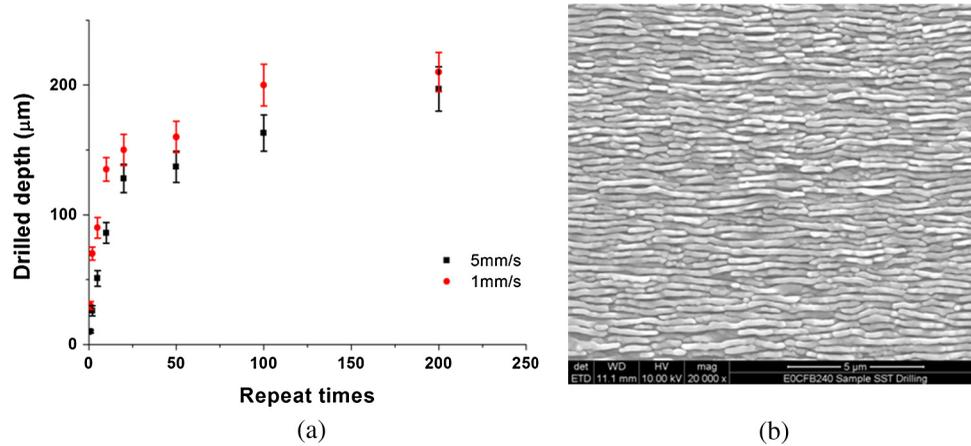
**Fig. 7** (a) Stainless steel drilling depths as function of repeat time using scanner. (b) SEM view of ripple structure on bottom of the drilled hole in stainless steel using fs fiber laser.
