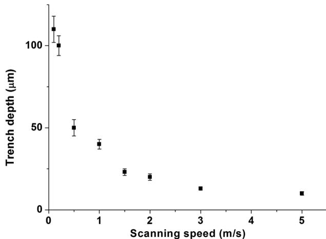
**Fig. 12** Titanium trench depth written using fs fiber laser for different speeds.
