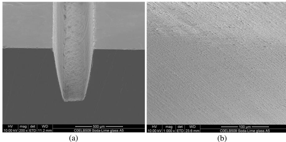
**Fig. 10** (a) SEM cross section view of soda lime glass trench written by using fs fiber laser and (b) SEM detail view of sidewall.
