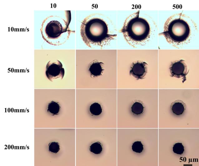
**Fig. 4** Microscope view of glass drilling using scanner with different speeds and repeat times.
