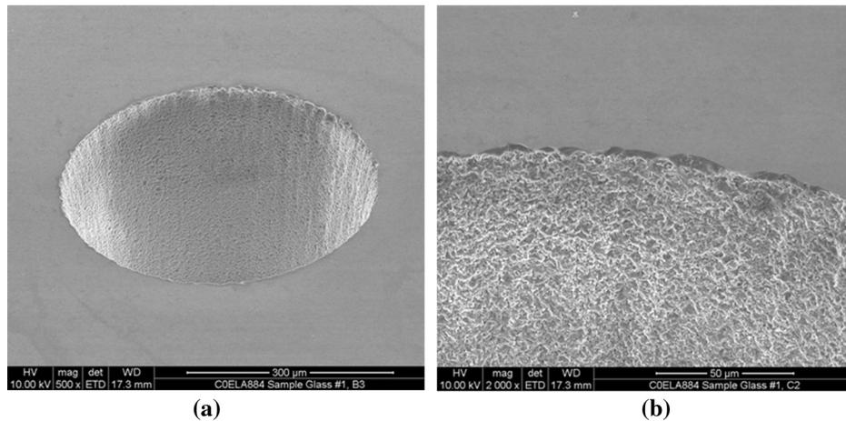
**Fig. 3** Scanning electron microscope (SEM) view of the drilled hole in soda lime glass using fs fiber laser: (a) Overview and (b) detail view of the hole edge and sidewall.
