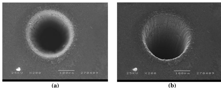
**Fig. 6** SEM view of deep hole drilling in stainless steel using fs fiber laser: (a) Top view and (b) side view of hole sidewall.
