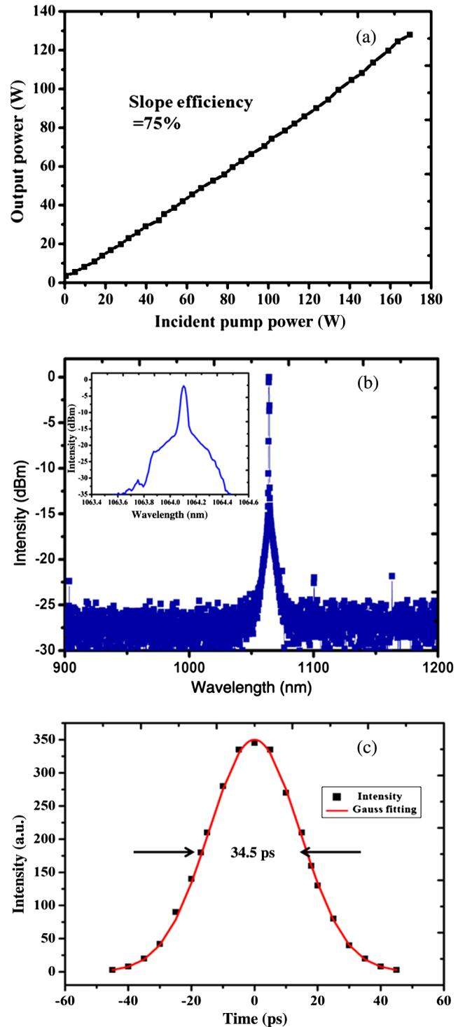
**Fig. 4** (a) Power scaling characteristics of the fiber amplifier, (b) optical spectrum obtained from amplifier at output power of 130 W (Inset shows the enlarged spectrum around the central wavelength), and (c) the pulse width at output power of 130 W.
