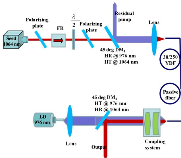
**Fig. 1** Schematic diagram of the high-power picosecond fiber amplifier based on a dual-cladding fiber.
