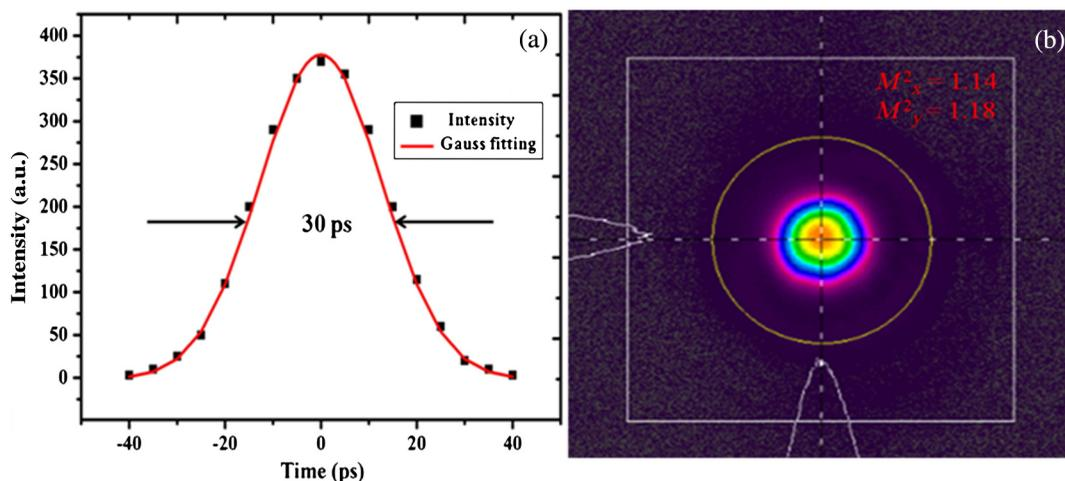
**Fig. 2** (a) The pulse width of the continuous wave mode locked (CWML) laser and (b) the beam quality profile at an output power of 2 W.
