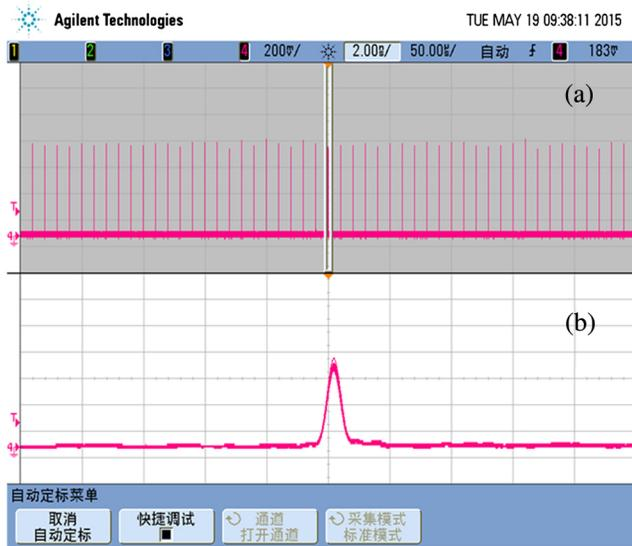
**Fig. 3** Typical CWML pulse trains at the repetition rate of 73.5 MHz in different time scales: (a) 50 ns/div and (b) 2 ns/div.
