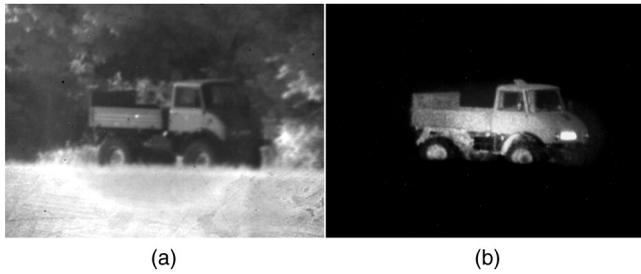
**Fig. 1** Passive SWIR (a) and active SWIR GV image (b) of a vehicle at a distance of 480 m (M400).
