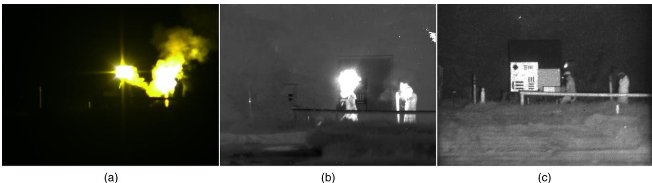
**Fig. 11** Synchronously captured images of a scene with two persons burning Bengal lights at a distance of 450 m. (a) Visual image. (b) MWIR image. (c) GV image (M506).
