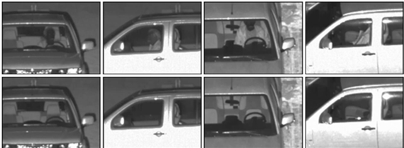
**Fig. 42** Cropped, active SWIR images at  $\lambda = 1.55 \mu\text{m}$  of a vehicle with person (top row) and without person (bottom row) at the wheel. The sensor elevation angle is 0 deg (first and second column) and 20 deg (third and fourth column). The target aspect angle is 0 deg (first and third column) and 90 deg (second and fourth column).
