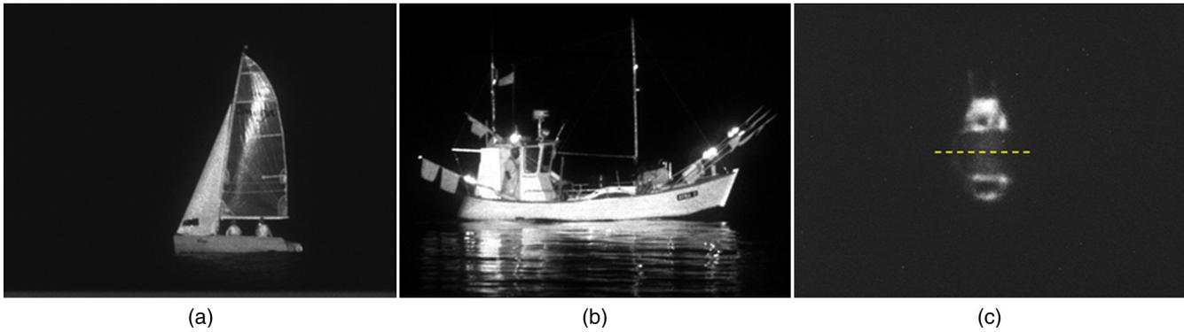
**Fig. 35** (a) GV images (M506) of maritime targets showing the capability for target segmentation, (b) indirect specular reflections, and (c) mirage effect at longer distances.
