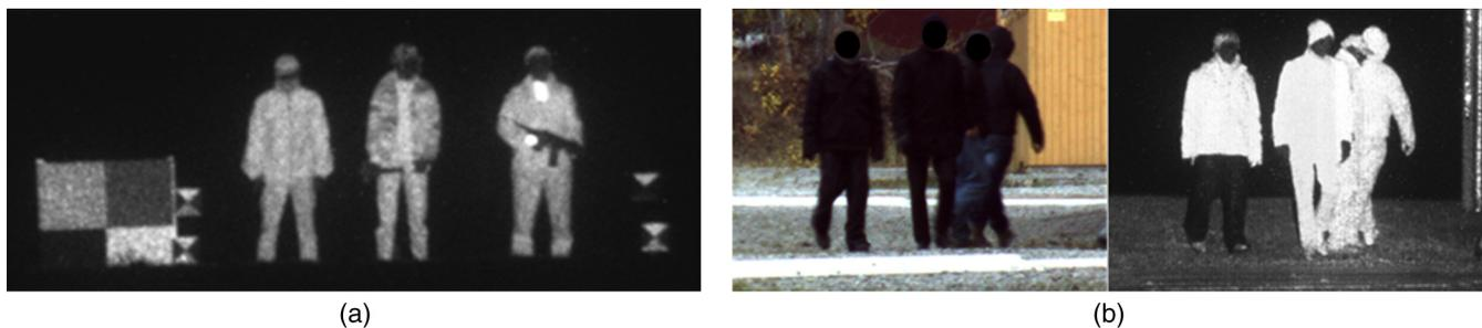
**Fig. 33** (a) GV image (M506) of four reference targets and three persons wearing different clothes for the purpose of measuring the laser reflectance of the clothes at  $\lambda = 1.57 \mu\text{m}$ . (b) Visual and GV image (M506) of persons with high reflecting clothes except one very low reflecting pair of trousers.
