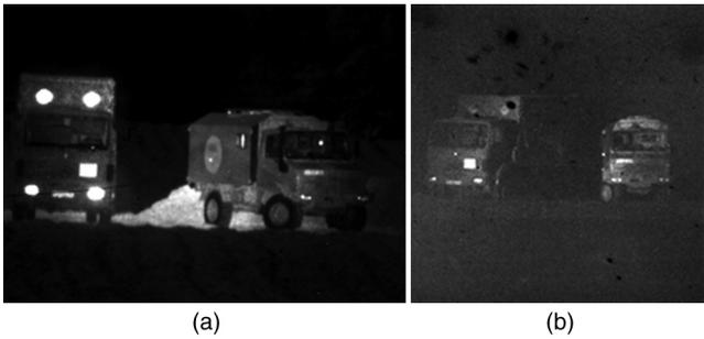
**Fig. 40** Monostatic (a, M400) and bistatic (b, M120) GV images of two vehicles at a distance of 600 m. The bistatic angle in the right GV image was 27 deg. The range gates were 590 to 640 m and 750 to 770 m, respectively.
