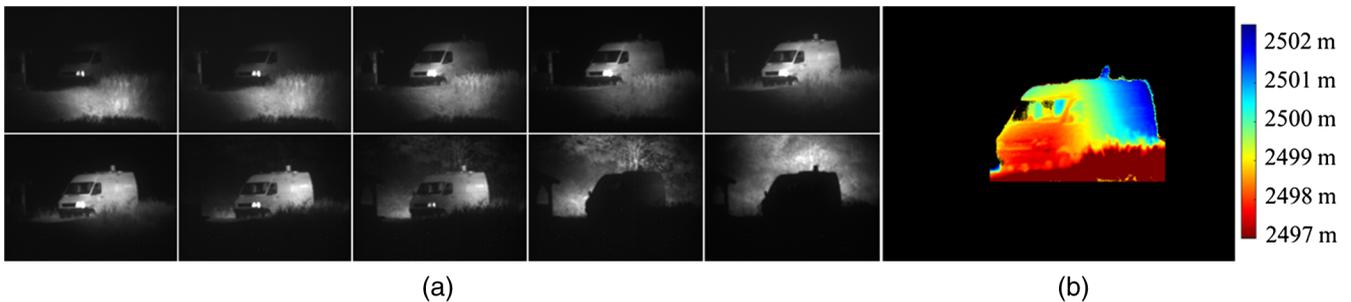
**Fig. 26** Precise 3-D reconstruction of a vehicle. (a) 10 GV images (M400) out of a sliding gates sequence consisting of 14 GV images with a gate shift step size of 1.5 m and a gate length of 9.75 m. For each image, the speckle reduction technique by wavelength diversity (compare Sec. 3.3) was applied. (b) Color-coded range image as result of the precise 3-D reconstruction.
