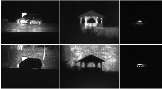
**Fig. 22** GV images (left and middle: M506, right: M120) of two vehicles and a cabin (top row) and corresponding silhouette images (bottom row). The distance of the vehicle in the left images is 215 m; the distance of the cabin in the middle images is 2455 m; and the distance of the vehicle in the right images is 7200 m.
