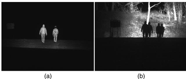
**Fig. 23** (a) GV image (M506) of two persons at a distance of 225 m and (b) corresponding silhouette image. Due to the bistatic system configuration, two silhouettes are visible for each person.
