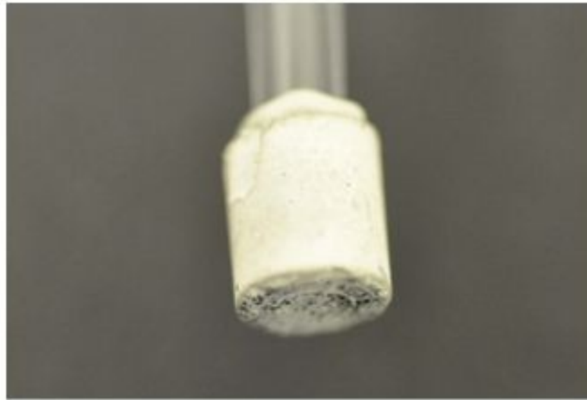
Figure 3. (a) Experimental setup for testing the nanoporous membrane. (b) The nanoporous alumina membrane.
