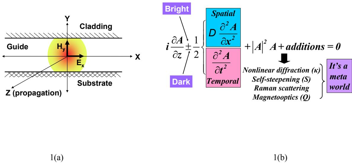
Fig.1(a) Nonlinear planar waveguide[central core is nonlinear; cladding and substrate are linear] supporting stable one-dimensional spatial solitons, experiencing diffraction along the x-axis and associated with an electric field component  $E_x$  and magnetic field component  $H_y$ .
