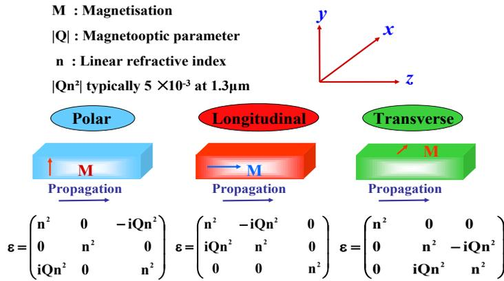
Fig.2 Typical magneto optic configurations
