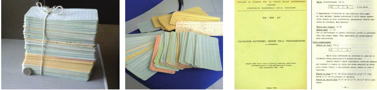
Fig. 1– Left: bundles of cards used for use with computer: old source program and cards with data for elaboration. Dimension reference: coin of one euro. Right: cover and one page of a course on Basic and Fortran languages
