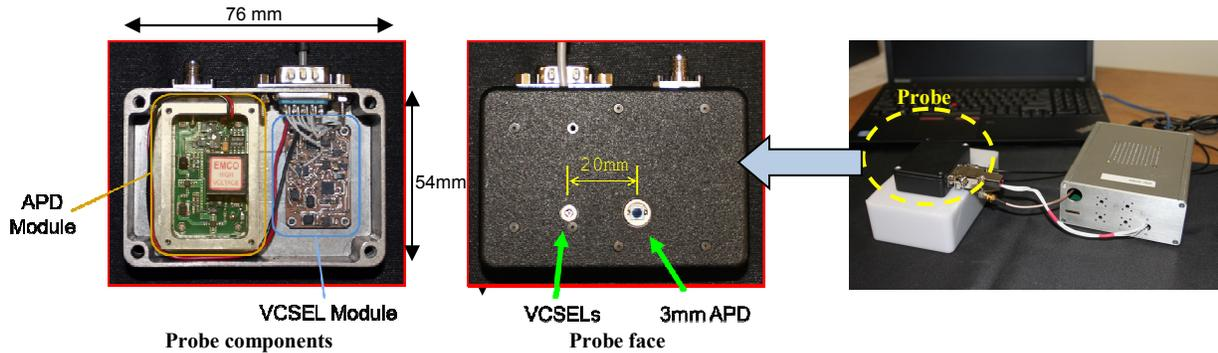
Figure 4: Prototype VCSEL-based FDPM module and integrated VCSEL/APD probe
