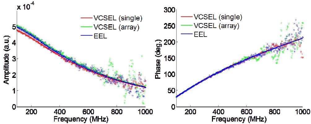
Figure 2: The calibrated amplitude and phase measured using FDPM through a tissue-simulating optical phantom ( $\mu_a=0.007 \text{ mm}^{-1}$ ,  $\mu'_s=1.01 \text{ mm}^{-1}$ ) at a source-detector separation of 22 mm.
