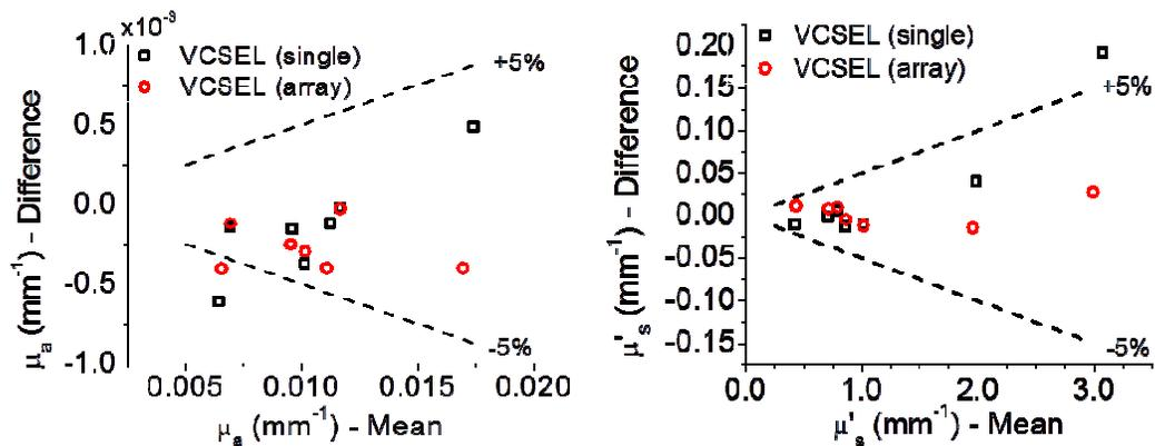
Figure 3: Bland-Altman plots which compare the optical properties recovered with the VCSEL devices (single and multiple aperture) with the standard EEL on 7 different phantoms with varying optical properties.
