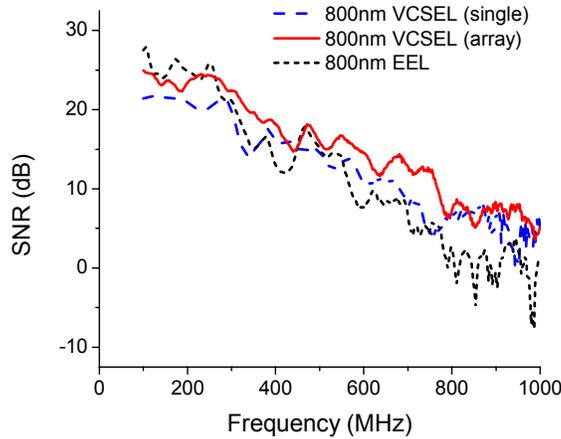
Figure 1: The modulation bandwidth of each laser measured with a high speed photodiode. The signal-to-noise ratio (SNR) was calculated by dividing the measured RF power by a prior dark noise measurement.
