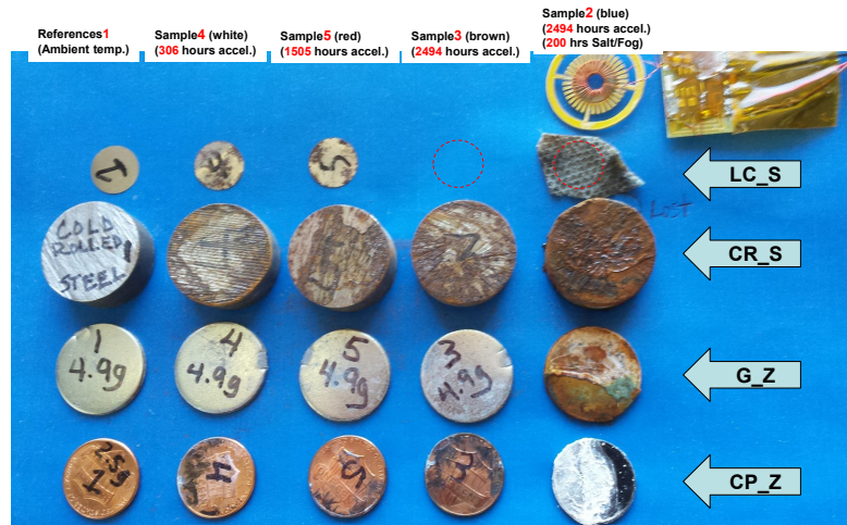
Figure 11. Photo of sensor at room temp and ambient relative humidity (rh), along with metal samples (after 306 to 2494 hours at 122 degrees F and 95.5 percent rh.)
