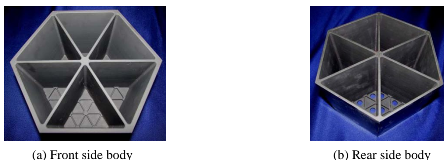
Fig. 8. Sintered bodies before grinding process
