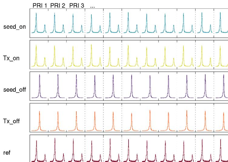
Fig. 9: Fringe pattern obtained in the operational sequence of the OPO pulses 'lambda\_Tx\_on' and 'lambda\_Tx\_off' and the two seed laser diodes 'lambda\_seed\_on' and 'lambda\_seed\_off', as well as the reference laser diode 'lambda\_ref'. Proc. of SPIE Vol. 10562 105620K-8
