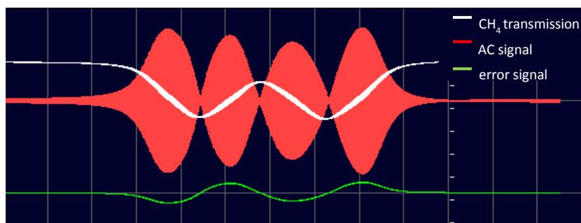
**Fig. 3:** Wavelength scan with additional current modulation by temperature tuning across the methane absorption feature showing the absorption, the AC photo receiver signal and the derived error signal for locking. The frequency span of the scan is about 10 GHz.
