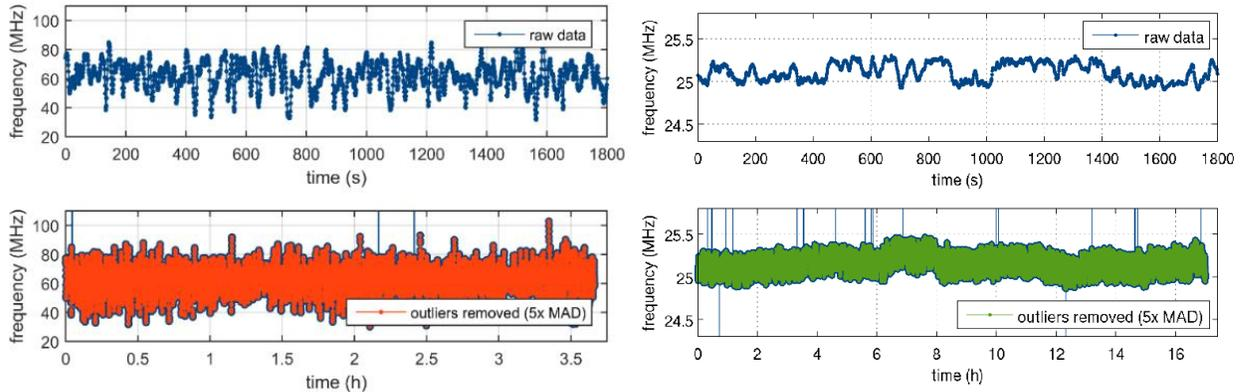
**Fig. 4:** Stability analysis of two independent absolute frequency references free running (left), locked (right). The upper parts are magnifications of the first half hour of the measurement. Please note the different vertical scaling between locked and unlocked data sets.
