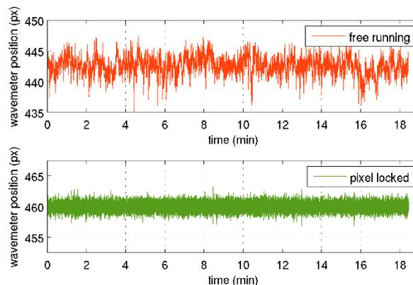
**Fig. 7:** Free running measurement of a DFB laser diode with the wavemeter and stabilization of a DFB laser diode a set pixel on the wavemeter.
