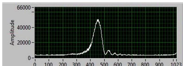
**Fig. 5:** Typical fringe produced by the Fizeau wedge measured with the CMOS line camera.
