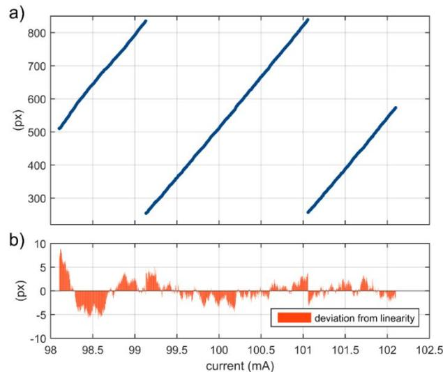
**Fig. 6:** Scan of the wavemeter by current tuning of the laser diode a) and characterization of the deviation from linearity due to pixel non-uniformity b) by applying a linear fit to the measurement data.
