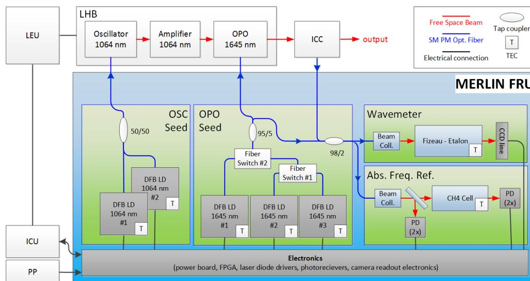
**Fig. 1:** Functional Diagram of the FRU and interfacing to the laser head box (LHB), instrument control unit (ICU), internal calibration chain (ICC) and primary power (PP).
