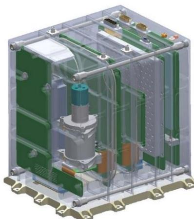
**Fig. 2:** Mechanical design of the FRU
