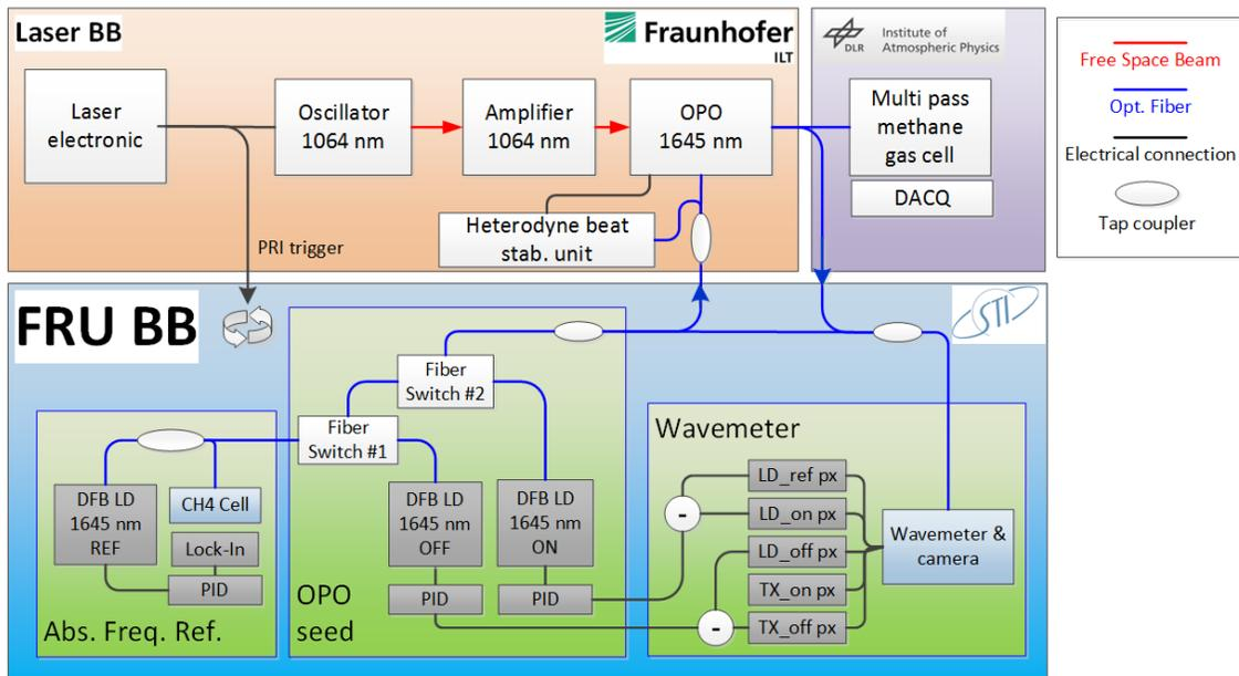
Fig. 8: Functional diagram of the test setup including the FRU breadboard (BB), the main laser breadboard developed by the Fraunhofer ILT and a multi pass gas cell for spectral purity measurements provided by the DLR IPA.
