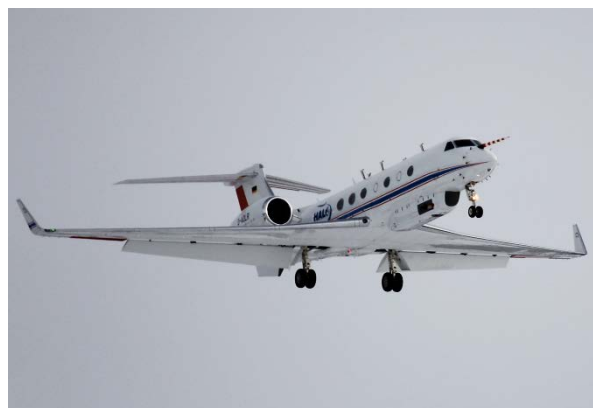
Fig. 1. Photographs of the airborne platforms carrying the DLR lidar systems. (a): DLR's Falcon 20 (D-CMET); (b): HALO, the German High Altitude Long Range research aircraft (D-ADLR). Here, the bellypod which can e.g. accommodate a radar antenna and an optical window aperture simultaneously is mounted below the aircraft's fuselage.
