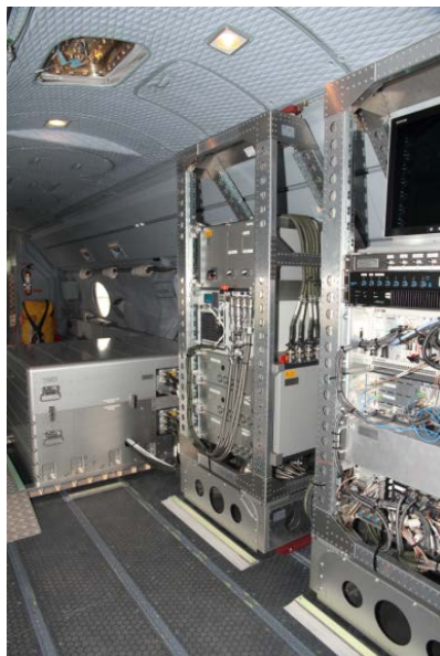
Fig. 7. CHARM-F, the combined CO 2 and CH 4 IPDA installed on-board the HALO research aircraft (a) and a narrow methane plume detected as an enhancement of the differential absorption optical depth (DAOD) along the flight path (b).
