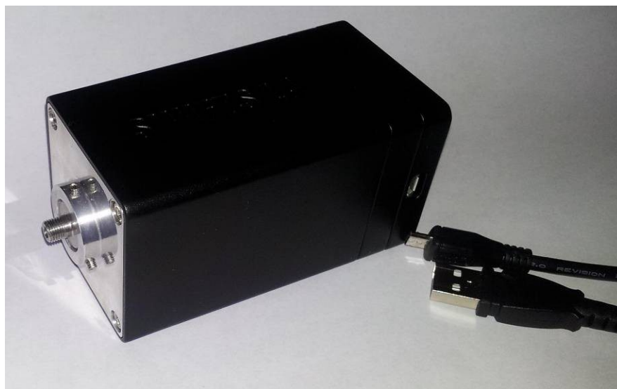
Fig. 3. : SWIFTS-LA, the 140g whole spectrometer detector allowing us to acquire digital images on an USB2 interface. The spectral resolution is 176pm at \lambda=762nm meeting the 200pm CARBON-SAT specification for Oxygen-B band.
